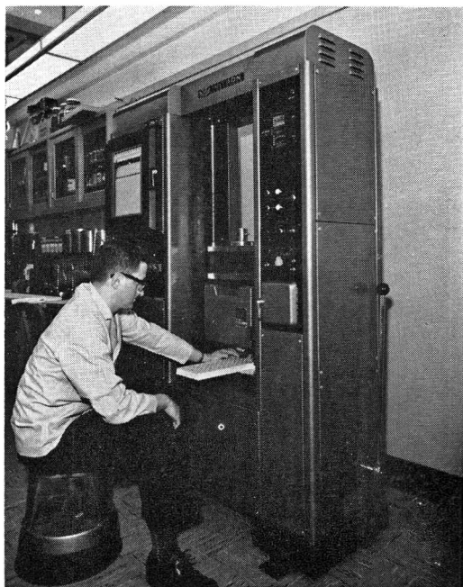
Fig. 3. Sheet of foam plastic board being punched in the Instron universal testing machine.
