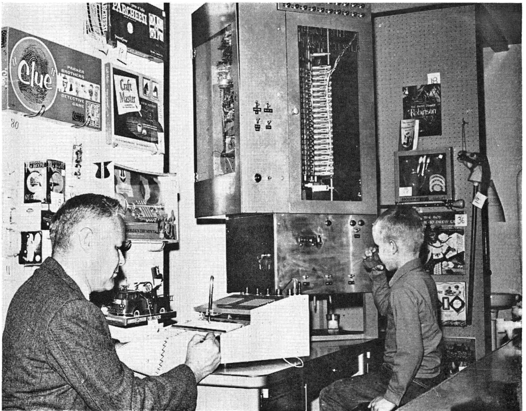
Fig. 4. Taste discrimination of young boy being determined with the aid of an automatic taste-testing machine. The recorder plots the successive concentrations of the taste solution that were tested.
