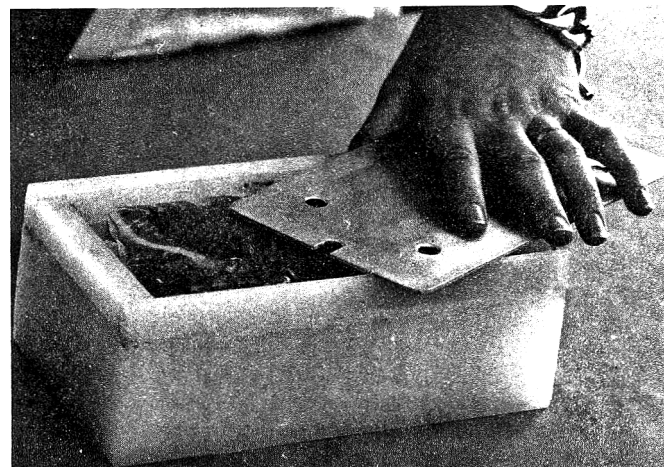
Fig. 2—Mould-electrode arrangement for RF-processing at 60 MHz; (top) cross section; (bottom) actual view.
