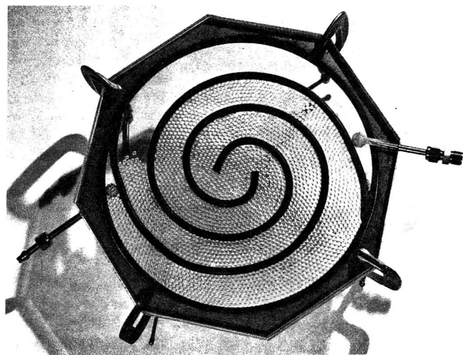
Fig. 1—Spheres in flow channel of transparent plastic mock-up (10.75-in.-diameter membrane area).
