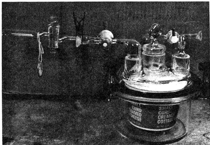
Fig. 1—Special glass container for studying the effect of selected gas atmospheres on the quality of stored cottage cheese. An ampule for gas sampling is shown attached at the left to 1 arm of the 3-way stopcock.
