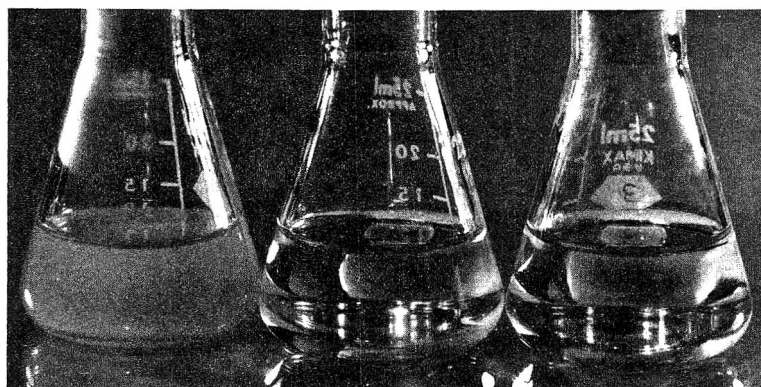
Fig. 1—Solubilization of water forming a one-phase system. Flask at left contains 10.0g orange oil + 0.57 ml water; center, 10.0g orange oil + 1.0g AOT; right, 10.0g orange oil + 1.0g AOT + 0.57 ml water.
