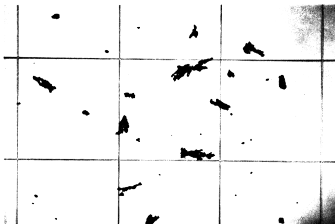
Fig. 1—Photomicrograph of metal particles isolated from a sample of enriched whole wheat flour on a micrometer disc with 1 mm squares.
