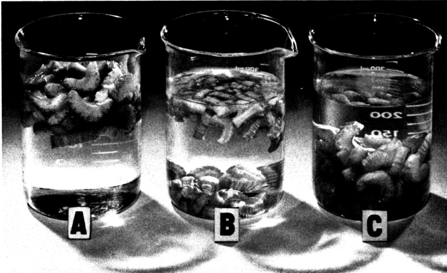
Fig. 3—Dehydrated celery, rehydrated: (a) Freeze dried; (b) Air dried; (c) Glycerated, air dried.
