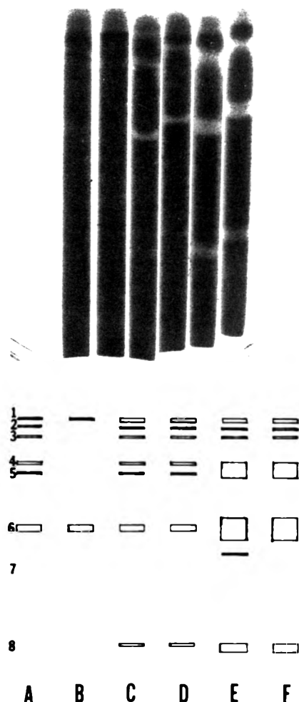
Fig. 1—Photographic and diagrammatic representation of polyacrylamide gels of extracts of cold stored tubers assayed for starch hydrolysis: (A) Kennebec, 1-hr assay at 30°C; (B) Monona, 1-hr assay at 30°C; (C) Kennebec, 5-hr assay; (D) Monona, 5-hr assay; (E) Kennebec, 18-hr assay; (F) Monona, 18-hr assay. Electrophoresis was at 3 ma/tube for 2.5 hr. Sample volume applied to the gel was 50 \mu l.
