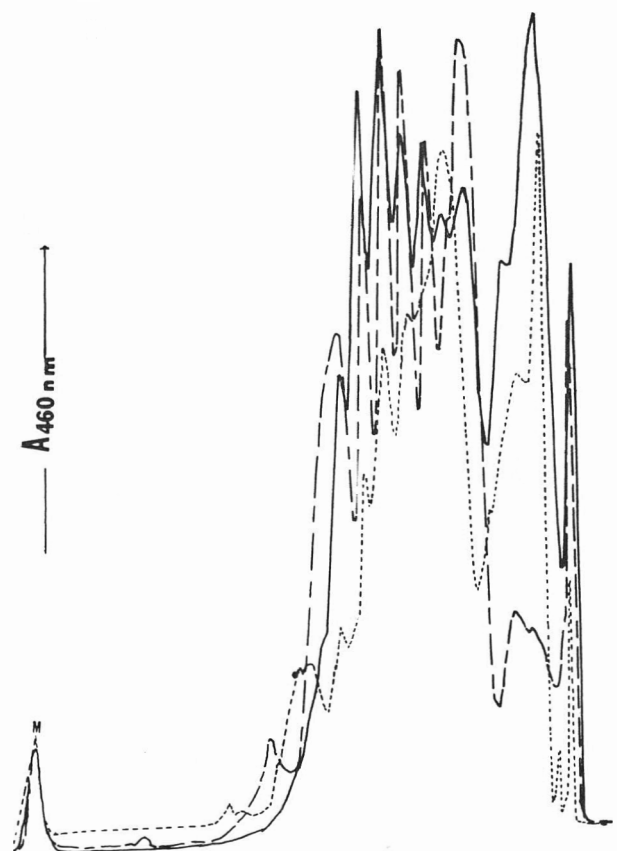
Fig. 5—Densitometric scans (460 nm, 50 mm/min) of polyacrylamide gels of 10 \mu l peroxidase extracts from spears stored at 20°C for 48 hr after harvest. Spears were divided into tip (---), mid (···) and butt (—) sections prior to extraction with medium containing 0.4M \text{CaCl}_2 . Marker (M) was approximately 8 cm from the origin of each gel.
