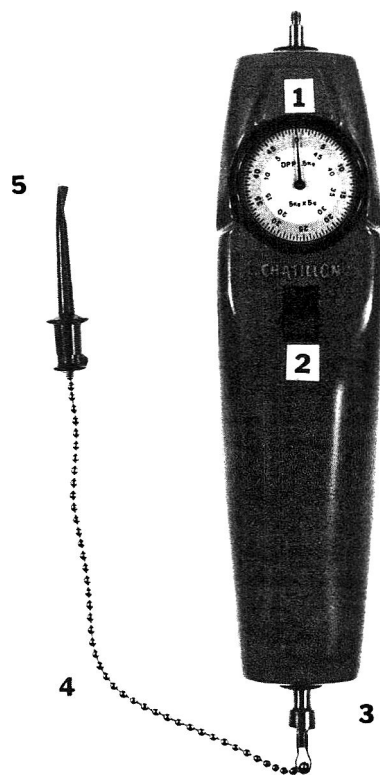
Fig. 1—The apparatus used for measuring the plucking force: (1) meter; (2) reset button; (3) 500g maximum load force gauge; (4) chain connecting spring to (5) the clamp that grasps the hair being tested.
