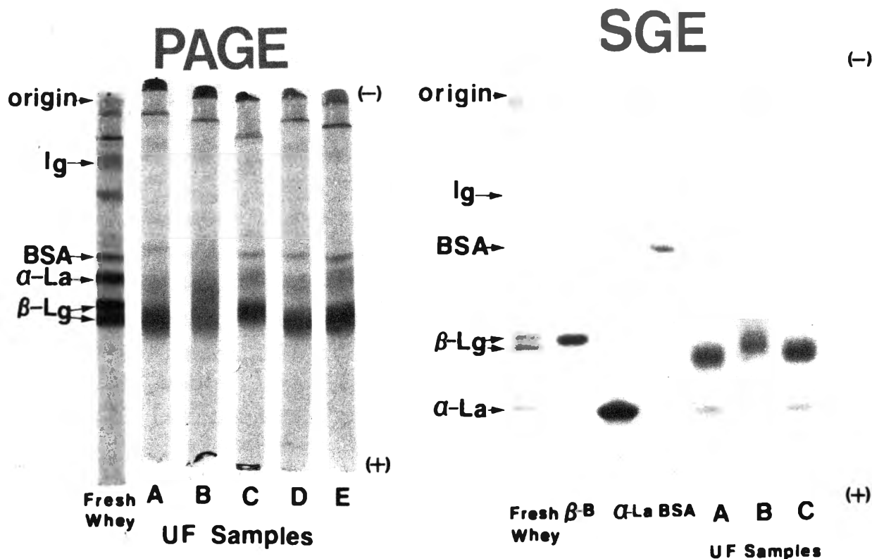
Fig. 2—Alkaline disc polyacrylamide gel electrophoresis (PAGE) and alkaline urea starch gel electrophoresis (SGE) patterns of fresh Cheddar whey selected whey protein standards (SGE pattern only) and selected lots of UF spray-dried sweet whey powders. Whey protein identification: \beta -Lg ( \beta -lactoglobulin); \alpha -La ( \alpha -lactalbumin); BSA (bovine serum albumin); and Ig (immunoglobulins).
