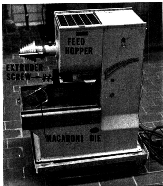
Fig. 1—La Parmigina laboratory model pasta extruder.
