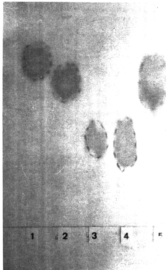
Fig. 6—Paper chromatograms of lactose hydrolysates by Scopulariopsis lactase: (1) glucose; (2) galactose; (3) lactose; (4) whey without enzyme; (5) whey with enzyme.
