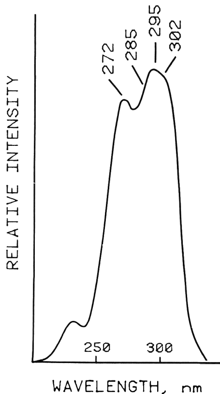
Fig. 7—Fluorescence excitation curve obtained from bulk concentrated orange juice for manufacturing imported by Florida processors with emission monochromator at 340 nm.
