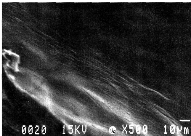
Fig. 8—Scanning electron micrograph of paper coated with 6.6 kg/ream corn zein, indicating increased surface uniformity compared to the 4.4 kg/ream coating level ( \times 500 ). White bar 10 micrometers.
