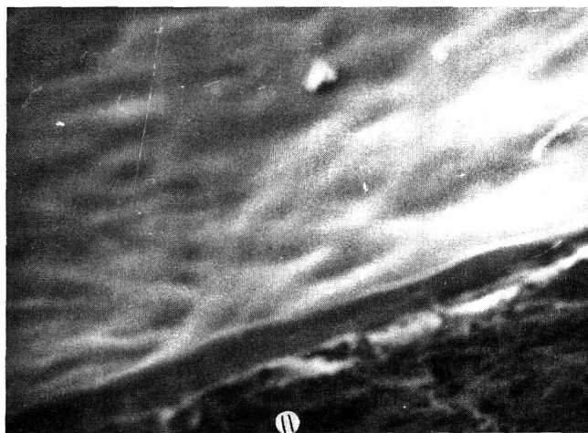
Fig. 7—Scanning electron micrograph of paper coated with 4.4 kg/ream corn zein, indicating a more uniform coating and less evidence of paper fibers at the paper/zein surface ( \times 200 ).
