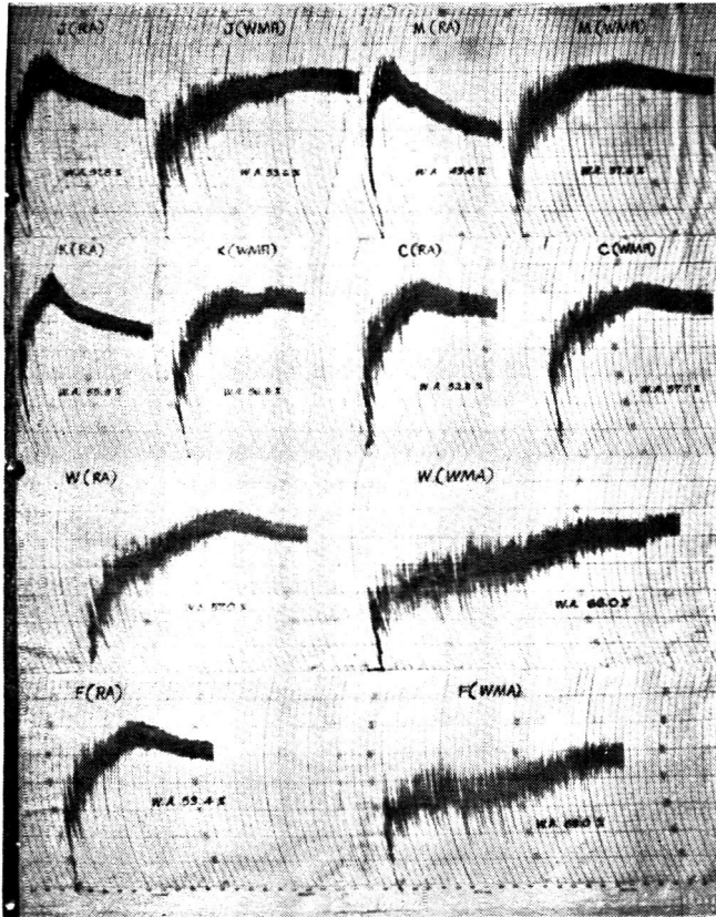
FIG. 1. Farinograms of resultant atta (RA) and atta (WMA)
