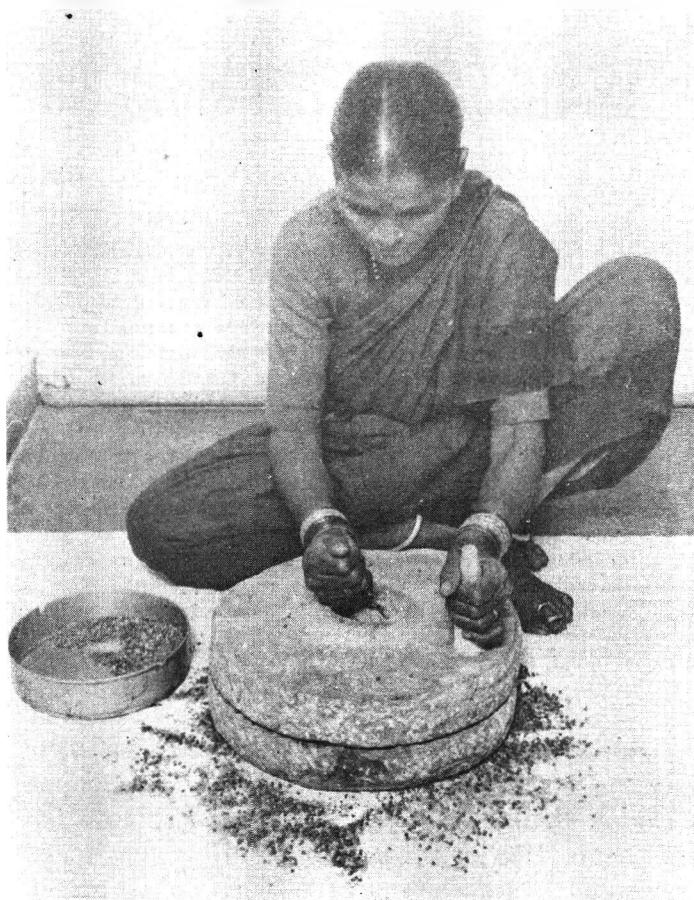
Fig. 2. Traditional method of dehulling pulses using stone chakki
