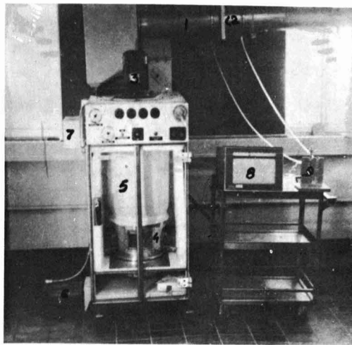
Fig 1. Manesty Petrie Fluid-bed dryer, 1. Air-flow pipe, 2. Orifice slide, 3. Fan motor, 4. Fluidizing bowl 5. Collecting bag, 6. Stirrer motor, 7. Ratiotrol 8. Speedomax recorder 9. Manometer
