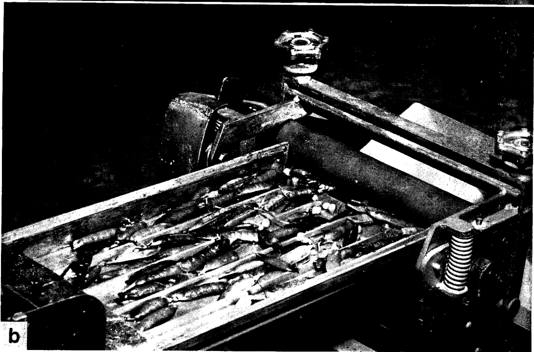
PLATE 1. C.S.I.R.O. pea sheller. (a) General view. (b) View showing vibratory conveyor, feed gap and shelling rollers.
