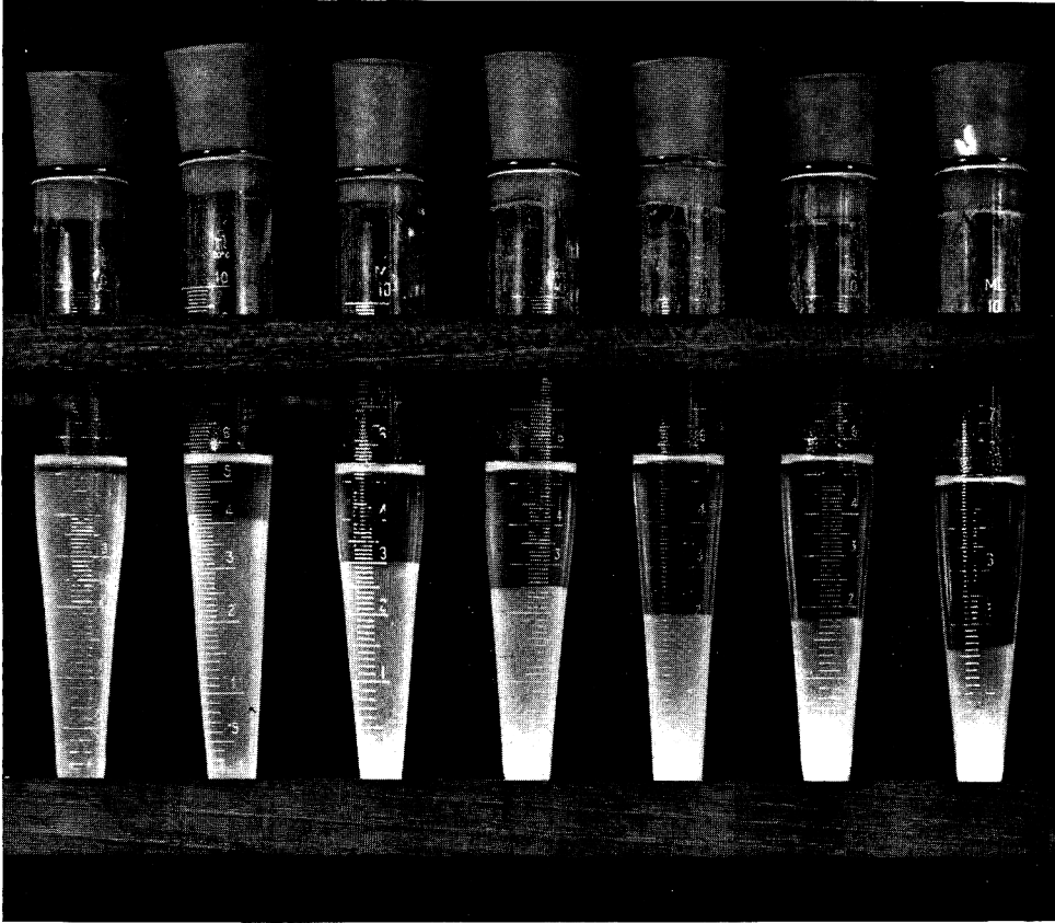
PLATE 3. Sedimentation volumes after centrifugation following swelling in DMSO. Left to right: untreated, 80°, 100°, 110°, 120°, 130° and 140°C heat treated flour.
