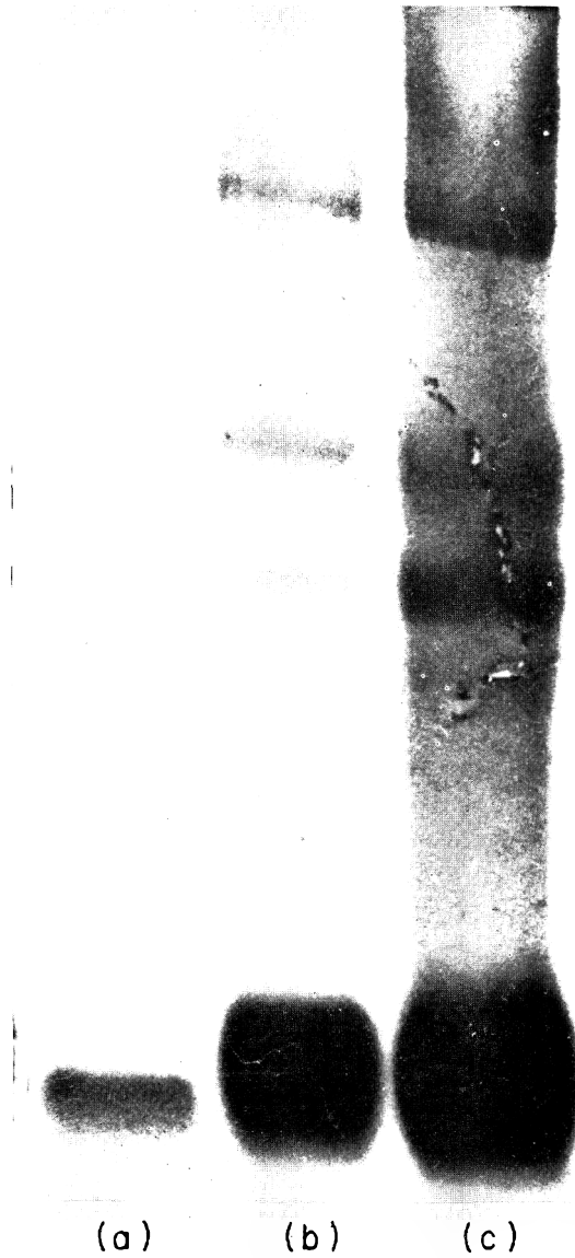
Plate 1. Polyacrylamide gel electrophoretic pattern of (a) porcine plasma, (b) supernatant formed on addition of 4% PEG, and (c) 8% PEG to plasma.
