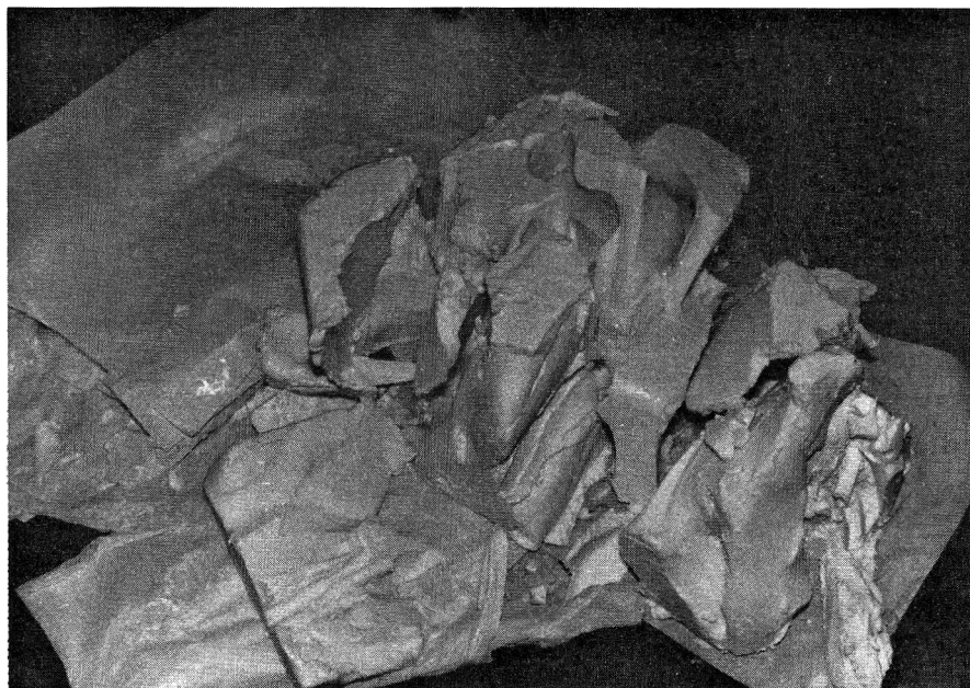
Figure 2. Photograph showing layering of butter emptied from a 25 kg carton which was filled from a pipe of a continuous buttermaking machine.
