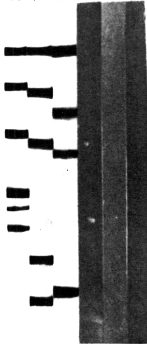
Figure 2. Polyacrylamide gel electrophoresis of Fraction I a proteins in 7.5% gels; a,d: 'Swedish Brown'; b,e: 'Sutter Pinto'; c,f: 'Bonus'. Gel portion, a,b,c was stained for protein (Mauer, 1971); gel portion d,e,f was stained specifically for TI's (Uriel & Berges, 1968).
