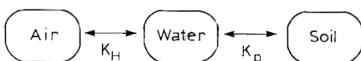
Fig. 1. Three-phase system. K_p is the soil-water partition coefficient, and K_H Henry's constant.
