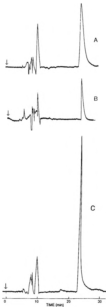
Figure 2. Chromatograms of corticosteroids analyzed individually and in mixtures. Column: 47 x 0.46 cm i.d., packed with 5- \mu m octadecylsilica material. Mobile phase: 35% aqueous acetonitrile; 0.5 mL/min. Detector: UV-VIS absorbance detector (240 nm, 0.005 AUFS). Solutes: (A) cortisone ( 10^{-6} M), (B) tetrahydrocortisol ( 10^{-3} M), (C) mixture of cortisone and tetrahydrocortisol.
