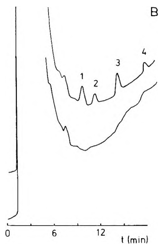
Figure 3. (A) The chromatograms of the blank and the spiked tap water after on-line preconcentration (500 ppt of benzylchloride (1) and chlorobenzene (2), 100 ppt of naphthalene (3) and biphenyl (4)). Sample volume: 100\text{ cm}^3 . (B) The chromatograms of the blank and the spiked river (Danube) water after on-line preconcentration (1 ppb of benzylchloride (1) and chlorobenzene (2), 200 ppt of naphthalene (3) and biphenyl(4)). Sample volume: 50\text{ cm}^3 . For the chromatographic conditions see Figure 1.
