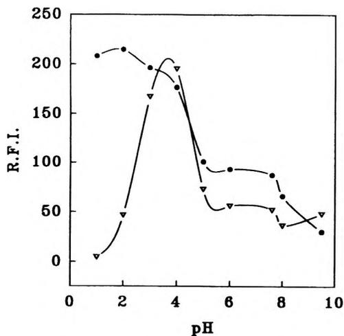
**Figure 3.** Influence of pH on the relative fluorescence intensity of (●) asulam and (▼) amitrole. Asulam  $8.7 \times 10^{-7}$  M and amitrole  $2.4 \times 10^{-4}$  M [FC] =  $3.6 \times 10^{-4}$  M.
