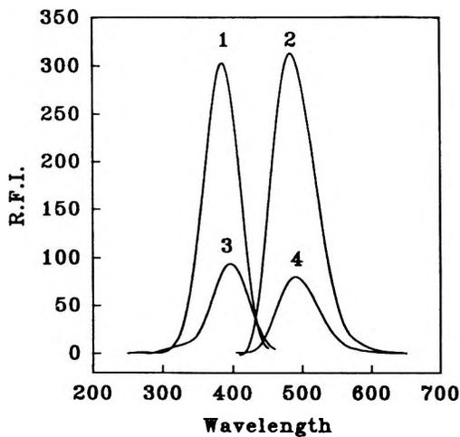
**Figure 2.** Excitation and emission spectra of FC derivatives of (1,2) amitrole and (3,4) asulam. Asulam  $8.7 \times 10^{-7}$  M and amitrole  $2.4 \times 10^{-4}$  M pH = 3; [FC] =  $3.6 \times 10^{-4}$  M.
