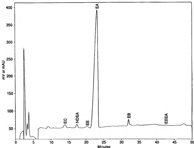
**Figure 3.** Typical chromatogram (monitored at 205 nm) obtained from the analysis of a commercial sample of erythromycin 2% topical solution. Details of chromatographic conditions are described in the experimental section and Table 1.
