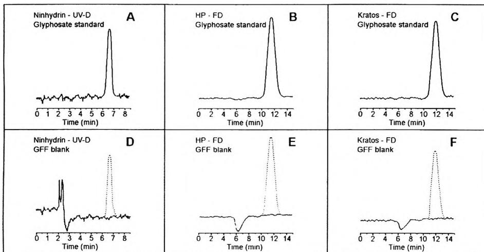
**Figure 4.** Representative chromatograms obtained from HPLC-PCR-ninhydrin (UV-D) and HPLC-PCR-fluorogenic (HP-FD and Kratos-FD) studies (glyphosate concentration injected 100 ng/50  $\mu$ L) glyphosate peak in field extracts is shown by a dotted line over blank chromatograms in D to F.
