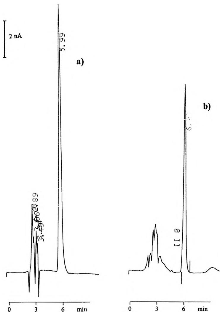
**Figure 2.** Comparative chromatograms of a) a standard solution of clopamide 5  $\mu\text{g/mL}$  and b) a diluted solution of a pharmaceutical formulation containing clopamide: Brineridine (-clopamide 10 mg, dyhydroergotaxine mesilate 0.58 mg, reserpine 0.1 mg and tartrazine 0.064 mg-).  $E = +1400$  mV; Flow rate: 1mL/min; Full current scale: 20 nA.
