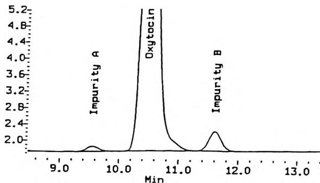
**Figure 1.** Typical chromatogram of the Resolution Solution.
