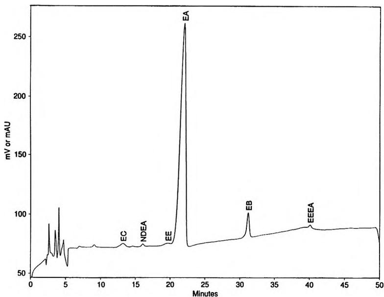
**Figure 2.** Typical chromatogram (monitored at 205 nm) obtained from the analysis of a commercial sample of erythromycin powder. Details of chromatographic conditions are described in the experimental section and Table 1.
