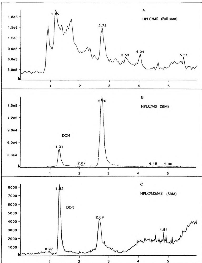
**Figure 3.** HPLC/MS analysis of corn feed spiked with 1 ppm levels of the three test compounds. A) Full-scan LC/MS TIC from the analysis of the supercritical fluid extract of the sample. B) SIM LC/MS analysis of the supercritical fluid extract of the sample. C) SRM LC/MS analysis of the supercritical fluid extract of the sample. See text for experimental details
