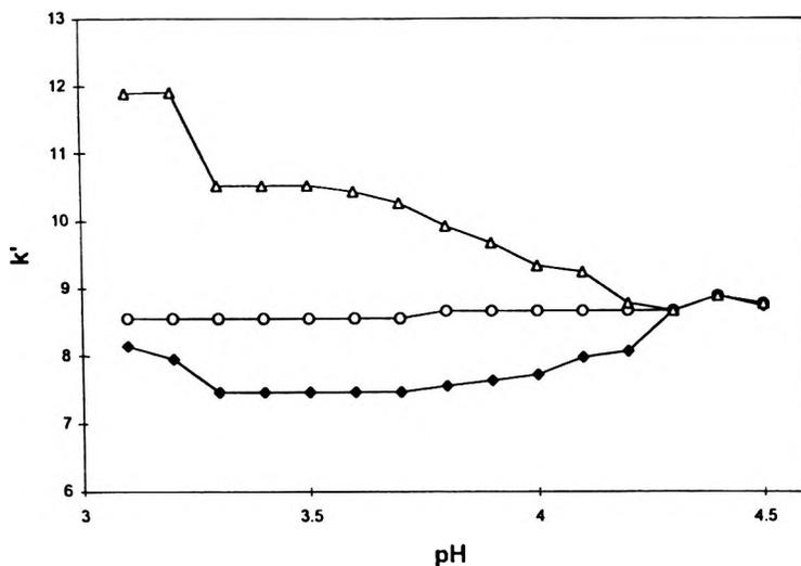
**Figure 2.** Effect of pH on  $k^*$ , where o = oxytocin, ● = impurity A and ■ = impurity B.
