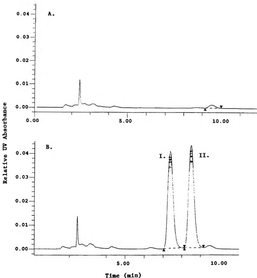
**Figure 2.** HPLC chromatograms of (A) blank murine plasma, (B) murine plasma containing the internal standard, costatolide (peak I: 335 ng) and (+)dihydrocalanolide A (peak II: 300 ng). Detector sensitivity, 0.001 AUFS.
