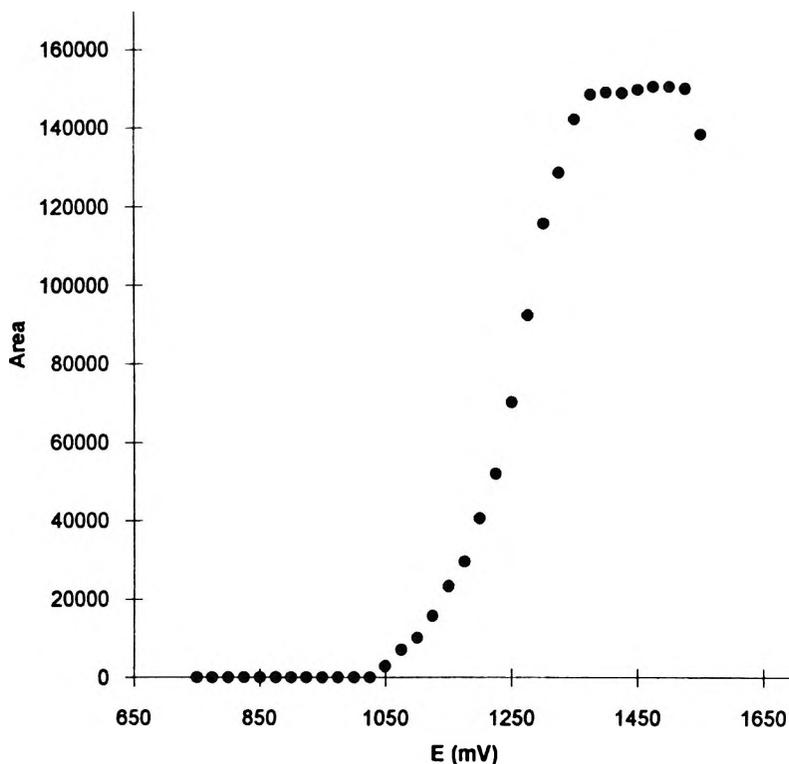
**Figure 1.** Hydrodynamic voltammogram of clopamide(●). Amount of drug injected: 100 ng in acetonitrile-water (35:65) containing 5mM NaCH<sub>3</sub>COO/CH<sub>3</sub>COOH, pH 5.5.
