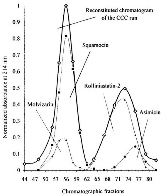
**Figure 2.** Chromatogram drawn from HPLC analyses of HSCCC fractions 44 to 82, showing the separation of molvizarin [1], squamocin [2], rolliniastatin-2 [3] and asimicin [4].
