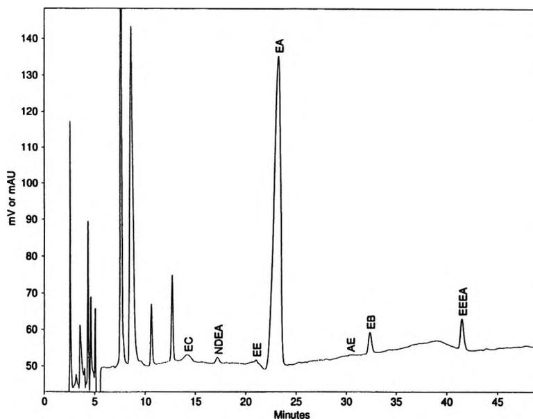
**Figure 5.** Typical chromatogram (monitored at 205 nm) obtained from the analysis of a commercial sample of erythromycin delayed-release tablet. Details of chromatographic conditions are described in the experimental section and Table 1.
