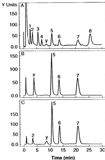
**Figure 2.** Chromatograms of  $\text{BH}_4$  and its analogues using IDA dual electrodes for EC detection followed by UV detection.
