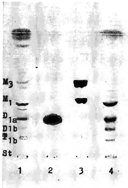
Figure 1. Thin-layer chromatogram of: (1) gangliosides after Sep-Pak procedure (test mixture added); (2) blood sugar (glucose); (3) GM1 and GM3 standards; (4) test mixture of bovine brain gangliosides; mobile phase: chloroform : methanol : sodium lactate = 55 : 40 : 10 (v/v/v); visualization by spraying with orcinol reagent.
