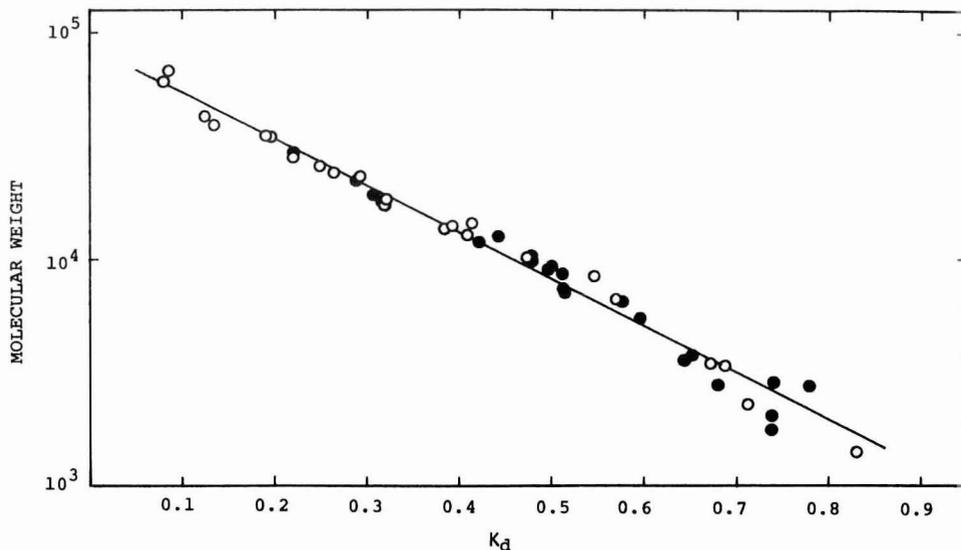
FIGURE 7 Plot of log molecular weight versus  $K_d$  of forty-five polypeptides and oligopeptides in 6 M guanidine hydrochloride and 0.05 M sodium phosphate buffer (pH 7.0). Charged samples were treated with 6 M guanidine hydrochloride and 0.05 M sodium phosphate buffer (pH 7.0) containing 0.3% 2-mercaptoethanol. The flow rate was 1.0 ml/min. Filled circles represent the data for CNBr fragments.
