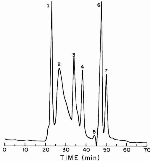
Figure 5. Elution curve of skim milk. Conditions as in Figure 4, 30  $\mu$ l injected.
