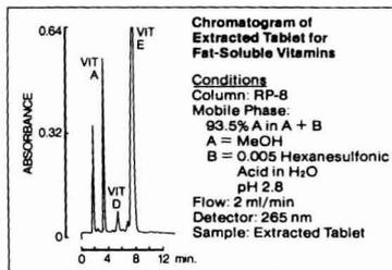
To assure that peaks were correctly identified, stopped-flow spectra were obtained—for example, only the peak eluting at about 5.5 minutes exhibits the strong absorbance at 266 nm which is characteristic of vitamin D.
