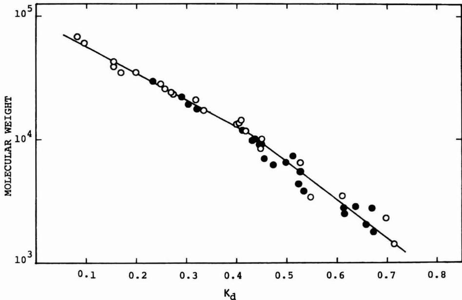
FIGURE 4 Plot of log molecular weight versus  $K_d$  of forty-five polypeptides in 0.2% SDS and 0.2 M sodium phosphate buffer (pH 7.0). The polypeptide samples were incubated and charged in a similar manner as described in Fig. 3. Filled circles represent the data for CNBr fragments.
