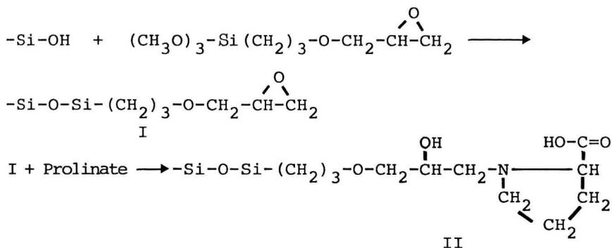
3-Glycidoxypropyltrimethoxysilane is bonded to silica gel in the first step. L-Proline (as sodium salt) is attached then to the epoxyd I in the second step to give product II. As a complexing agent Cu(II) ions were used. The loading of the support with metal ions can be carried out before packing and "in situ" after packing. Better results were achieved by "in situ" loading.
