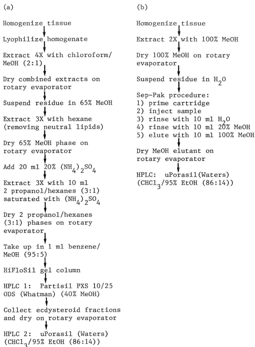
FIGURE 1. Extraction and purification of ecdysteroids for HPLC analysis using (a) solvent partition and (b) Sep-Pak C18 cartridges
