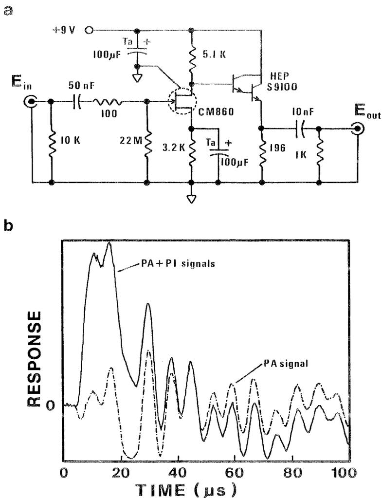
Figure 2: (a) Low noise preamplifier with R-C input coupling for polar mobile phases. The CM860 JFET is the four lead version of the 2N6550 JFET (Teledyne Crystallonics, Cambridge, MA).
