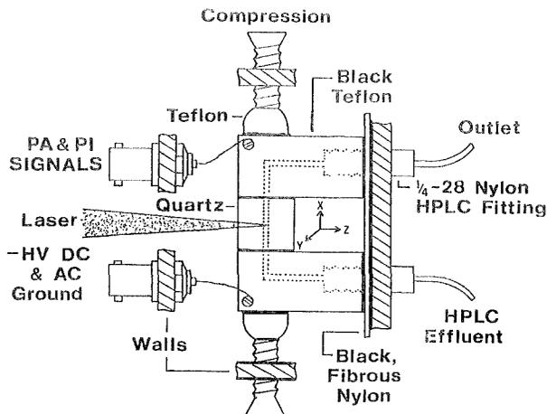
Figure 1: Schematic of the crystalline quartz cube HPLC flow cell.
