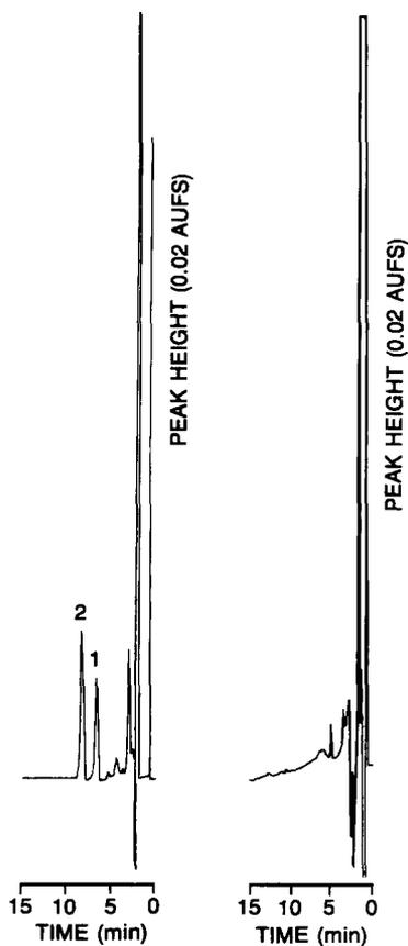
FIGURE 3 (i) Representative chromatogram of cefoperazone (1) and cephalothin (2) in serum. (ii) Representative chromatogram of a blank serum sample.
