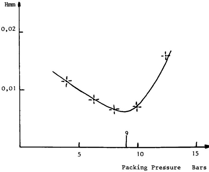
Figure 1. Variation of HETP vs packing pressure
