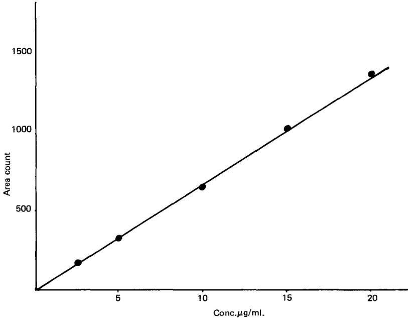
Figure 2. Calibration curve for Pirenzepine from urine under the present chromatographic conditions.
