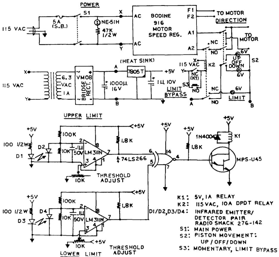
Figure 4. Control circuitry for pump. All resistors are 1/4 W, 5% unless otherwise specified.
