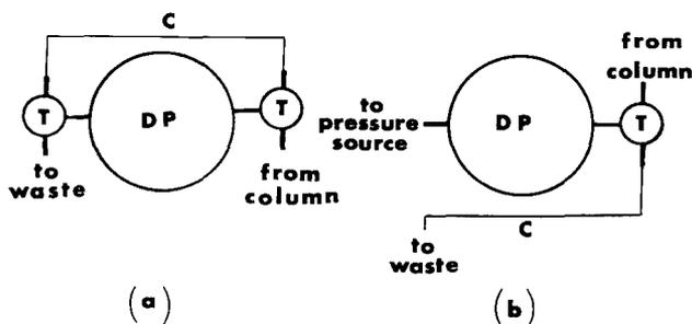
Figure 1. Two modes of detector configuration. T : zero dead volume tee; C : capillary; DP : differential pressure transducer.
