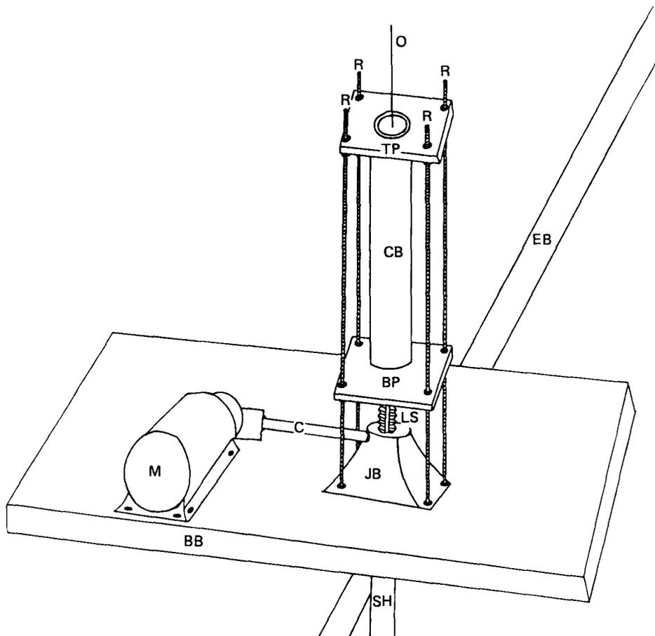
Figure 2. High pressure syringe pump. M : motor; C : coupling, motor shaft to worm shaft; JB : jack body; LS : lifting screw; SH : lifting screw housing; BB : baseboard; EB : edge of workbench; CP : syringe barrel; BP : bottom retaining plates; TP : top retaining plate; R : threaded support rods; O : pump outlet.
