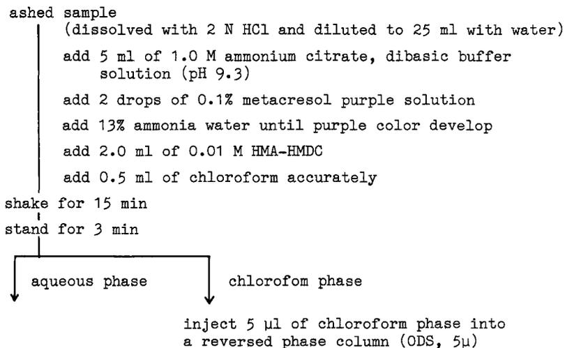
FIGURE 5 Recommended Extraction Procedure for the Determination of Cd, Ni, Pb, Zn, Cu, Co, Hg and Bi in Biological Samples
