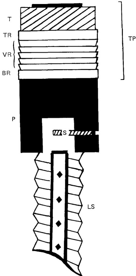
Figure 3. Details of the piston. T : teflon disc; TR : top, V-ring set; VR : v-rings (5); BR : bottom, V-rings set; P : stainless steel body of piston; TP : threaded portion of P; LS : lifting screw; S : retaining screw attaching lifting screw to piston. Diamonds in the lifting screw key slot indicate where numerals are engraved.
