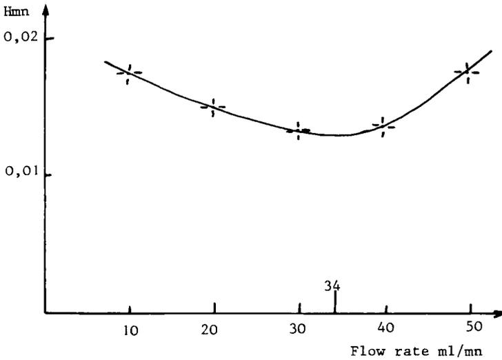
Figure 2. Variation of HETP vs flow rate
