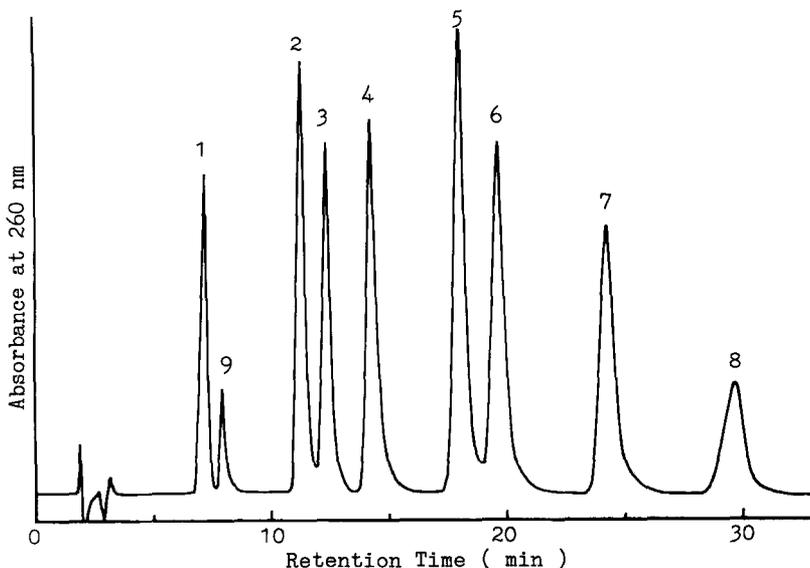
FIGURE 8 Typical Chromatogram of Metal-HMDC Chelates
