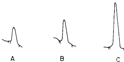
FIGURE 1. Typical densitometer scans of 200 ng (A) and 400 ng (C) standard chlorpyrifos zones and fortified tap water extract (B) chromatographed on the same layer. The sample represented 86.7% recovery (300 ng theoretical) when its area was interpolated from the calibration curve calculated from all standards chromatographed in parallel with the sample. An attenuation setting of X5 was used.
