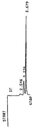
Figure 1. An HPLC chromatogram of a water sample at 102 \mu\text{g/L} using the reverse phase C18 system. (Peak of interest = 3.679 minutes)
