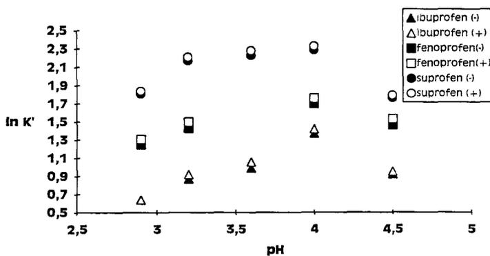
FIGURE 3 Plots of  $\ln k'$  vs pH values of the acetate buffer for a series of 2-APAs enantiomers. Chromatographic conditions as on figure 1.
