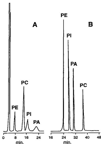
**FIGURE 2.** Separations of mixtures of PL standards (A) by HPLC-UV under isocratic elution on a  $\beta$ -CDS column; (B) by HPLC-ELSD under gradient elution on a SI column. Mobile phases: (A) [hexane-ISP-ETOH-water/5 Mm TMAP(Ph 6.3)] (35: 32.7: 26.8: 5.5); (B) See EXPERIMENTAL for gradient solvent systems.
