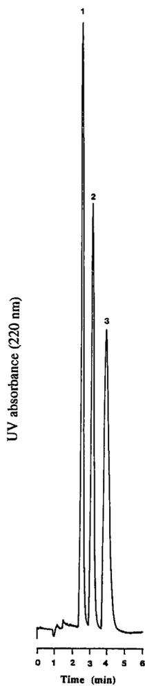
**Figure 1:** HPLC chromatogram of a standard solution containing  $10.0\mu\text{g}\cdot\text{ml}^{-1}$  of morphine (1), 6-acetylmorphine (2) and diamorphine (3).
