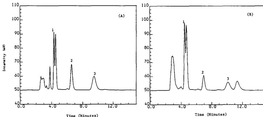
Figure 6. Chromatograms of injections # 15 (A) and # 280 (B) of chiral separation of methocarbamol enantiomers.
