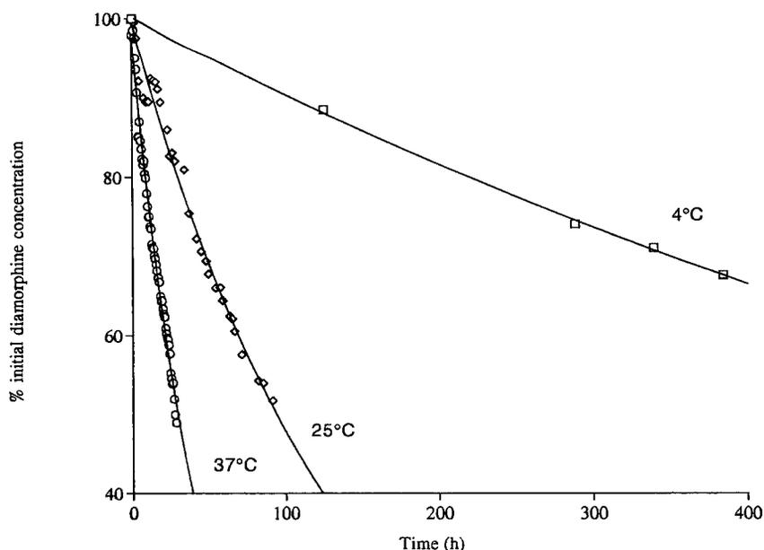
Figure 2: The effect of temperature on the stability of diamorphine in pH 7.4 buffer.
