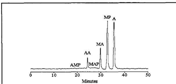
**Figure 2:** Chromatogram of aminocarb and its metabolites by FD. Retention times set to match with UVD values.
