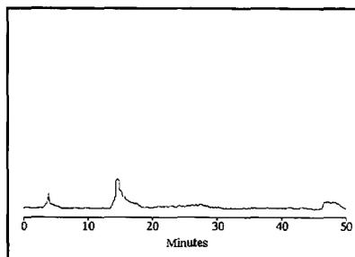
**Figure 5B:** Chromatogram of stream water blank by FD, after column cleanup.
