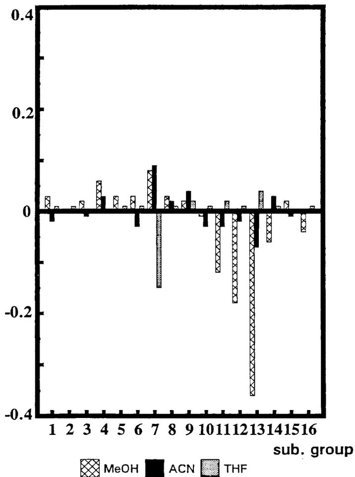
**Figure 3:**  $\Delta \log k'_{\text{experimental}} - \Delta \log k'_{\text{calculated}}$  difference values for various substituent groups calculated from the  $\Delta \log k' - \Delta \log k'$  correlation for the cyano - C-18 column pair (eqs. 4-6 in Table VII).
