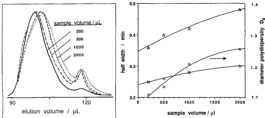
**FIGURE 4.** Effect of sample volume on the separation of a cadmium sulfide sol (10mM  $\text{Cd}(\text{ClO}_4)_2$ , 60mM polyphosphate, 1mM  $\text{H}_2\text{S}$ ).
