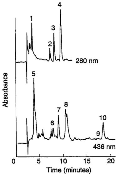
Figure 3. Chromatogram of a typical serum sample. Peak identification: 1=retinol, 2= $\Gamma$ -tocopherol, 3= $\alpha$ -tocopherol, 4= $\alpha$ -tocopheryl acetate, 5=lutein and zeaxanthin, 6=cryptoxanthin, 7=echinenone, 8=lycopene, and 9= $\alpha$ -carotene, 10= $\beta$ -carotene.
