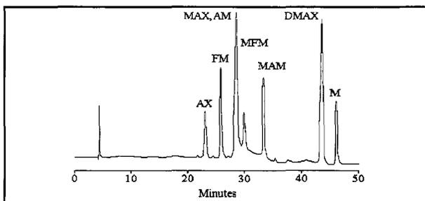
**Figure 3:** Chromatogram of mexacarbate and metabolites by UVD with RT (min): M=46.11; MFM=30.02; MAM=33.11; FM=25.85; AM,MAX=28.86; DMAX=43.43; AX=23.02.
