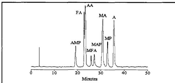
**Figure 1:** Chromatogram of aminocarb and metabolites by UVD with RT (min): A=35.94; MFA=25.83; MA=30.90; FA=23.80; AA=24.22; MP=32.44; MAP=27.12; AMP=19.06.
