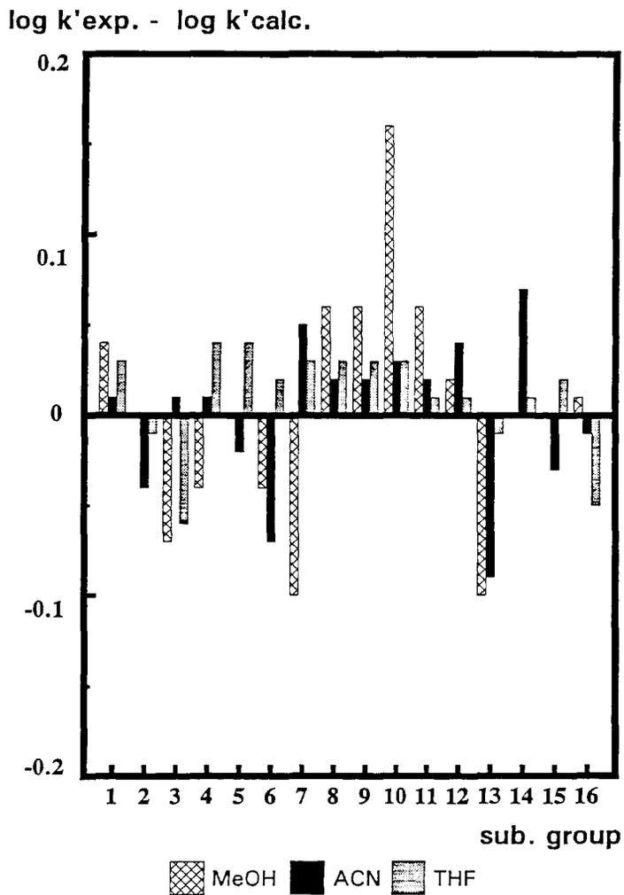
**Figure 2:**  $\Delta \log k'_{\text{experimental}} - \Delta \log k'_{\text{calculated}}$  difference values for various substituent groups calculated from the  $\Delta \log k' - \Delta \log k'$  correlation for the phenyl - C-18 column pair (eqs. 1-3 in Table VII).
