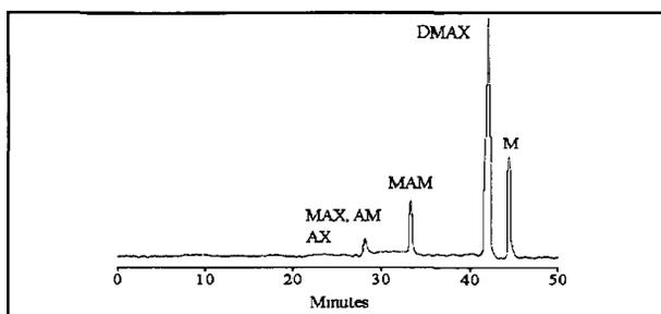
**Figure 4:** Chromatogram of mexacarbate and its metabolites by FD. Retention times set to match with UVD values.
