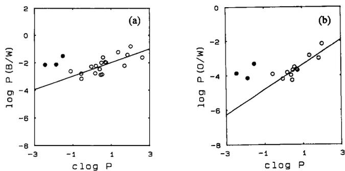
Fig. 2. A correlation of measured log P values (a) in n-butanol/water (b) n-octanol/water with clog P. The chelates GdL (where L = DTPA-BMA, DO3A and DO3MA and plotted by solid points) do not fall on the line.
