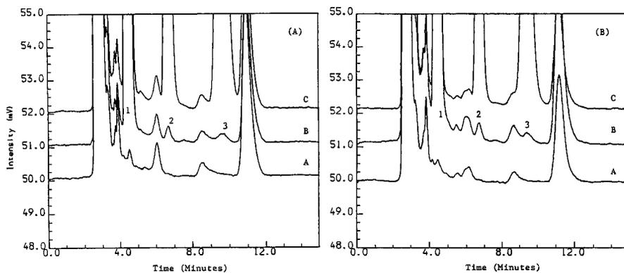
Figure 3. Chromatograms of chiral separation of methocarbamol enantiomers in human plasma on two lots (A and B) of Spherisorb CN and Chiralcel OD column.
