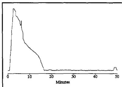
**Figure 5A:** Chromatogram of stream water blank by UVD, after column cleanup.
