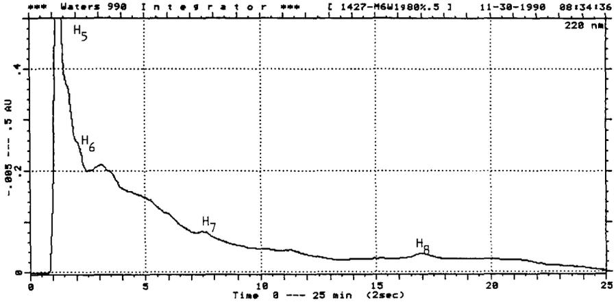
Fig. 5. Chromatogram of oil extract M6W/20D. Detection at 220 nm.
