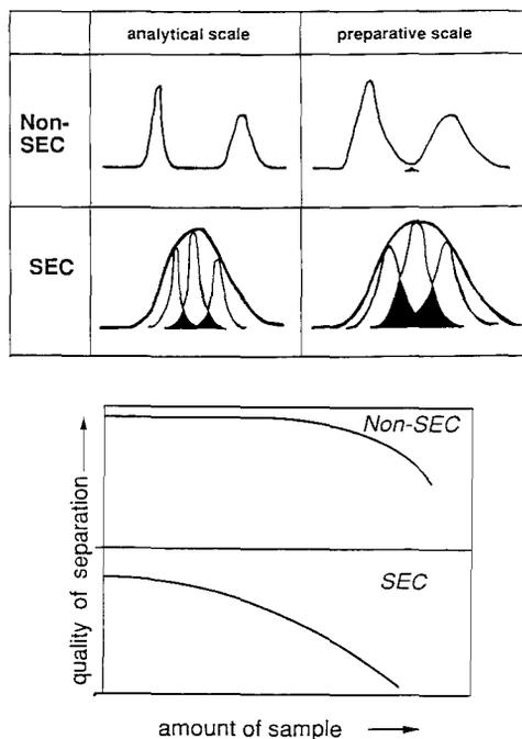
**FIGURE 1.** The effect of overloading in chromatography: Schematic comparison of non-SEC-methods and SEC with broad distributions. The overlapping areas of the peaks are marked in black. The SEC peak has to be considered as an overlay of numerous elemental chromatograms of one particular size. The graph on the bottom describes in principle the quality of the separation (size distribution or product purity, respectively) as a function of the amount of sample.
