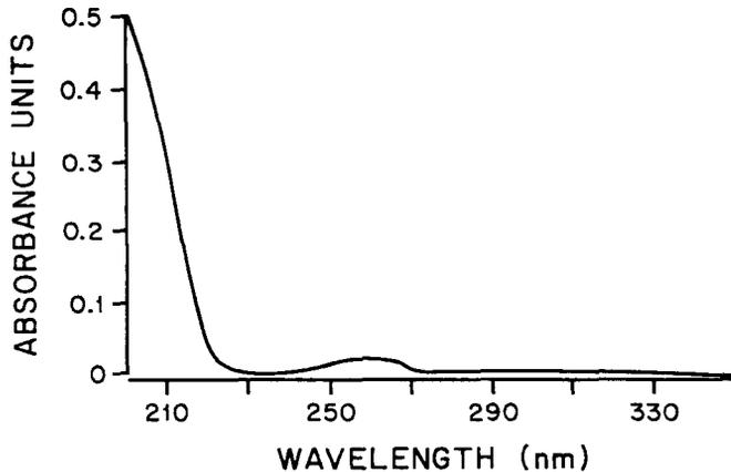
Fig. 2. Ultraviolet absorbance spectrum obtained with a concentration of 111  $\mu\text{g/ml}$  of fluconazole.
