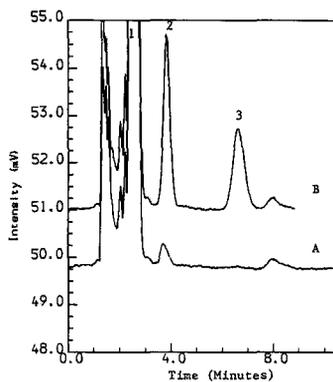
Figure 4. Chromatograms of chiral separation of methocarbamol enantiomers in human plasma on a Chiralcel OD column alone.
