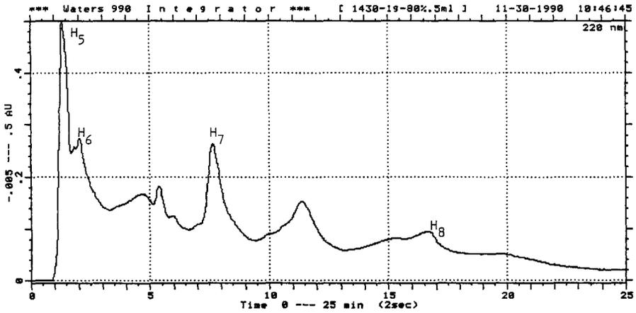
Fig. 6. Chromatogram of oil extract M6W/20D after 898 Km. Detection at 220nm.
