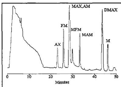
**Figure 7A:** Chromatogram of water by UVD, fortified with mexacarbate and its metabolites each at 0.5 µg/mL.
