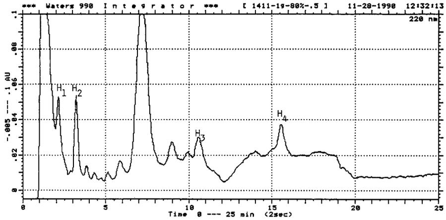
Fig. 3. Chromatogram of oil extract MT 16p, detection at 220 nm.
