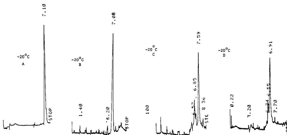
**Estriol resolved at subambient temperature (-20°C) by HPLC. Chromatograms shown are A: Standard Estriol (E<sub>3</sub>) peak with retention time  $t_{RE3}$ = 7.10; B: Normal Amniotic fluid, C: Down's Syndrome; D: Trisomy-18. Detection of E<sub>3</sub> = 280 nm.**
