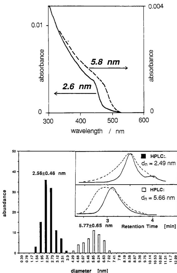
**FIGURE 8.** Bottom: Size distribution of two cadmium sulfide sols after preparative HPLC fractionation obtained by transmission electron microscopy (smaller particles: 5mM  $\text{Cd}(\text{ClO}_4)_2$  /30mM polyphosphate and 5mM NaHS mixed 4 : 1 (v/v); bigger particles: 10mM  $\text{Cd}(\text{ClO}_4)_2$ , 60mM polyphosphate, 10mM  $\text{H}_2\text{S}$ ). The inset shows the normalised analytical chromatograms of the diluted original samples and of the fraction analysed by TEM.
