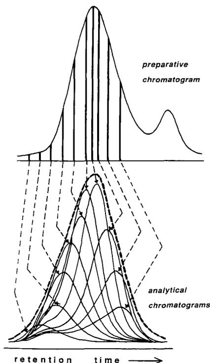
**FIGURE 2.** Characterisation of a preparative fractionation of a cadmium sulfide sol. Preparative chromatogram (**top**). The small peak is due to polyphosphate. Ten fractions (marked in black) were collected and re-injected in the analytical SEC (**bottom**), dashed line: diluted original sol, peak height adapted). Both time scales are different. Chromatographic conditions are given in the experimental part.
