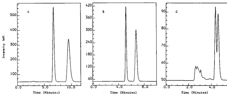
Figure 2. Chromatograms of chiral separation of unextracted methocarbamol (A), guaifenesin (B), and I.S. (C).
