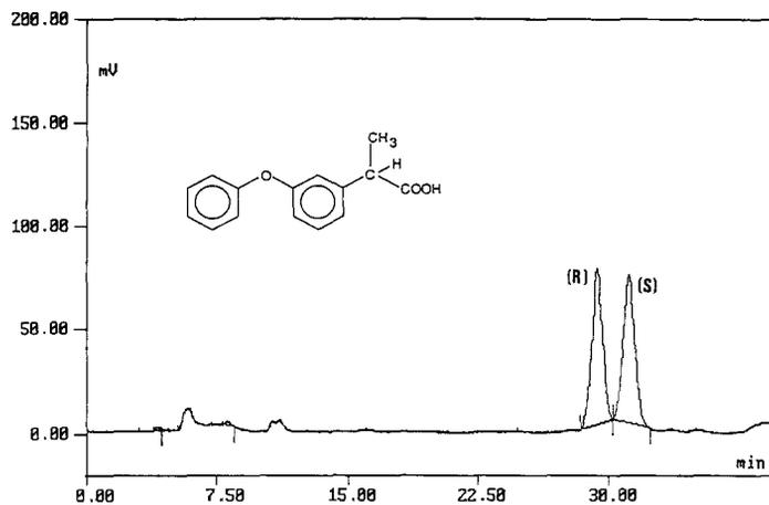
FIGURE 2 Chiral separation of (R)- and (S)- fenopropfen enantiomers. Chromatographic conditions: 0.05 M potassium acetate buffer (pH 4.6) / acetonitrile (60:40 v/v); flow-rate 80  $\mu$ l/min;  $\lambda$ , 254 nm.
