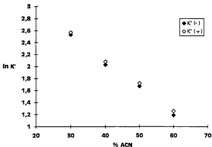
**FIGURE 1** Plot of  $\ln k'$  vs acetonitrile content of the mobile phase for naproxen enantiomers. Chromatographic conditions: column, 50 x 0.1 cm i.d.; buffer, 0.05 M potassium acetate at pH 4.0; flow rate, 80  $\mu$ l / min; UV detector set at 254 nm.
