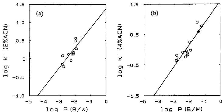
Fig. 4. Plot of  $\log k'$  (a) in 2% and (b) 4% acetonitrile vs.  $\log P$  in n-butanol/water.
