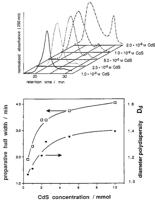
**FIGURE 5.** Effect of sample concentration on the separation of 500 $\mu$ l cadmium sulfide sol from  $[\text{Cd}(\text{ClO}_4)_2] : [\text{polyphosphate}] : [\text{H}_2\text{S}] = 10 : 60 : 1$  (details in the text).
