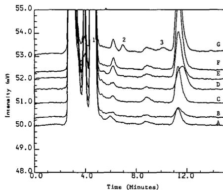
Figure 5. Chromatograms of screening six lots of blank control human plasma for the chiral separation of methocarbamol enantiomer.
