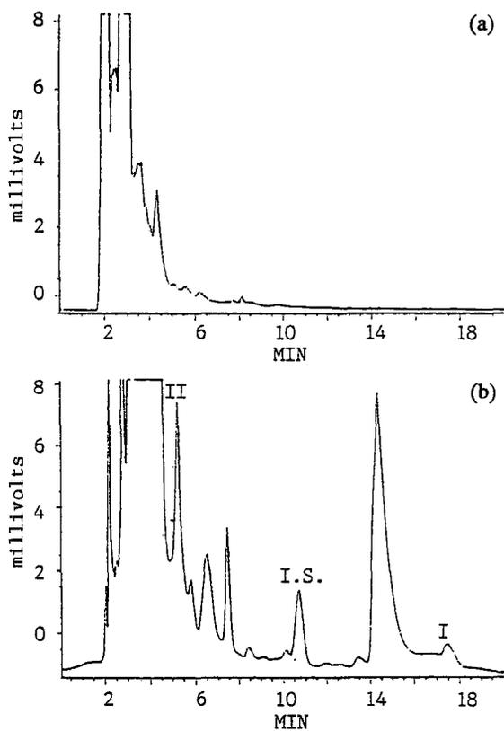
Figure 3. Representative chromatograms from (a) blank urine and (b) urine sample 1 hr after oral dose of 20 mg/kg of I to a dog. See experimental for chromatographic conditions. The estimated concentration (free + conjugated) of I and II was 3.1  $\mu\text{g/ml}$  and 4.2  $\mu\text{g/ml}$ , respectively. I.S. = Internal Standard
