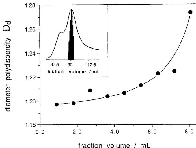
**FIGURE 7.** Effect of fraction volume on the separation of 200 $\mu$ l cadmium sulfide sol (10mM Cd(ClO<sub>4</sub>)<sub>2</sub>, 60mM polyphosphate, 10mM H<sub>2</sub>S). Diameter polydispersity of the main fraction as a function of the fraction size. The inset shows the preparative chromatogram and the size of the fractions. Experimental details are explained in the text.
