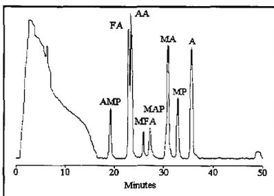
**Figure 6A:** Chromatogram of water by UVD, fortified with aminocarb and its metabolites each at 0.5 µg/mL.
