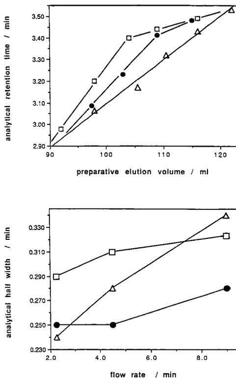
**FIGURE 3.** Effect of flow rates on the separation of a cadmium sulfide sol (5mM  $\text{Cd}(\text{ClO}_4)_2$ , 30mM polyphosphate, 1mM  $\text{H}_2\text{S}$ ).
