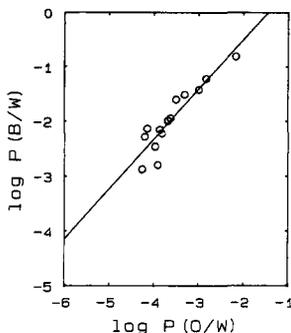
Fig. 1. Plot of  $\log P_{n\text{-butanol/water}}$  vs.  $\log P_{n\text{-octanol/water}}$ .
