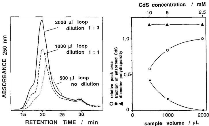
**FIGURE 6.** Comparison of the combined effects of sample concentration and sample volume on the separation of colloidal cadmium sulfide. The original sol was prepared from 10mM  $\text{Cd}(\text{ClO}_4)_2$ , 60mM polyphosphate, 10mM  $\text{H}_2\text{S}$ . The sample volumes were 500 $\mu\text{l}$ , 1000 $\mu\text{l}$  and 2000 $\mu\text{l}$ , but the latter two were diluted 1:1 and 1:3, respectively with water.
