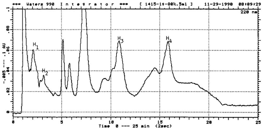
Fig. 4. Chromatogram of oil extract MT 16p after 1392 Km. Detection at 220 nm.
