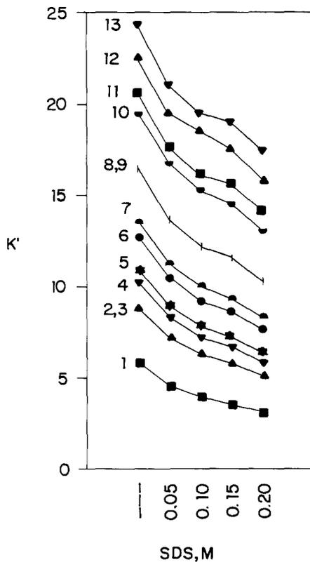
**FIGURE 1.** Effect of SDS concentration on the capacity factors of PAHs. The PAHs identified are indicated in Table 3.
