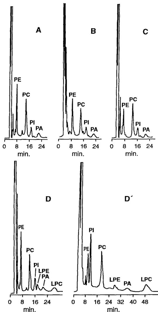
**FIGURE 4.** HPLC-UV-CDS separations of PL components in a commercial soybean lecithin sample (A) and experimental soybean lecithin samples (B, C, and D). HPLC-UV-CDS separation (D') of PL components was obtained from sample (D). Mobile phases: (A, B, C, and D) same as in FIGURE 2A. ; (D'), [hexane-ISP-ETOH-water/5 Mm TMAP(Ph 6.3)] (25: 38.5: 31.5: 5.0).
