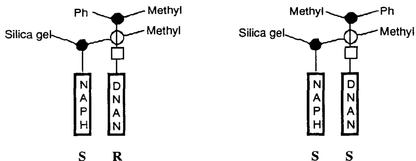
Figure 3. Schematic representation for the two diastereomeric (R,S)- and (S,S)-complexes between the 3,5-dinitroanilide derivative of racemic \alpha -phenylpropionic acid and (S)-CSP 2. See the caption of Figure 1 for the meaning of solid circle, empty circle and empty square symbols.
