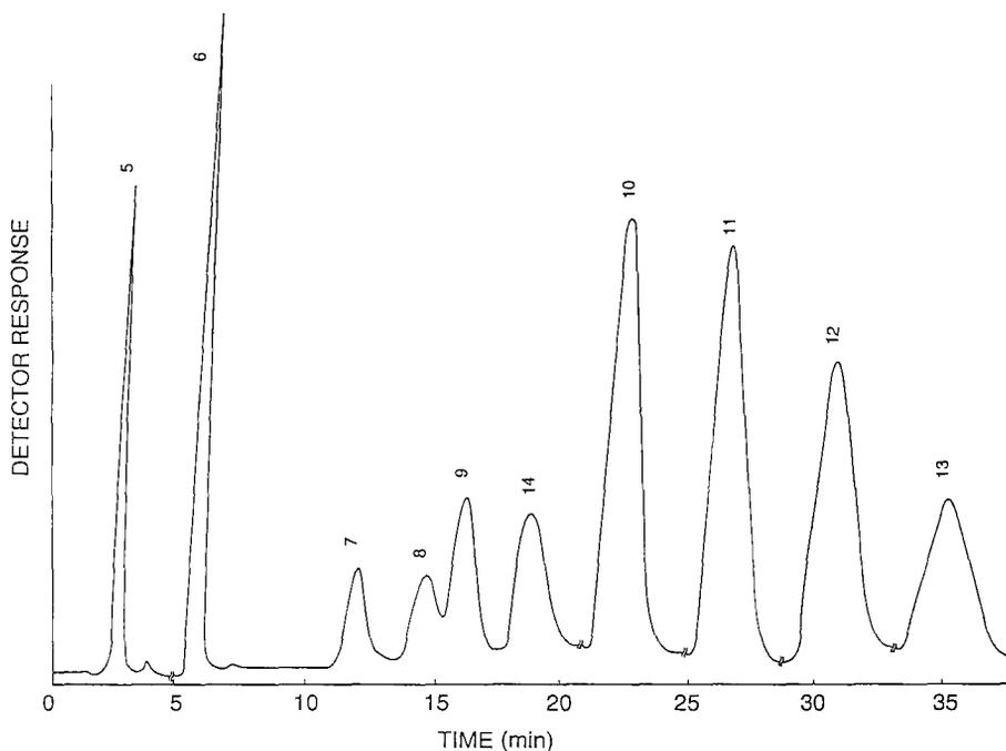
FIGURE 5. Chromatogram of ten metabolites of B[a]P obtained with MeOH:H<sub>2</sub>O (80:20) with 1.7 mM  $\gamma$ -CD. The full names of the compounds are given in the footnote of Table 1.
