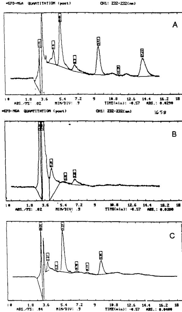
Fig. 4. (A) : Chromatographic analysis of urine spiked with cocaine=14.10 min, benzoylecgonine=5.37 min and the internal standard nalorphine=9.41 min(5 ng/ $\mu$ l).
