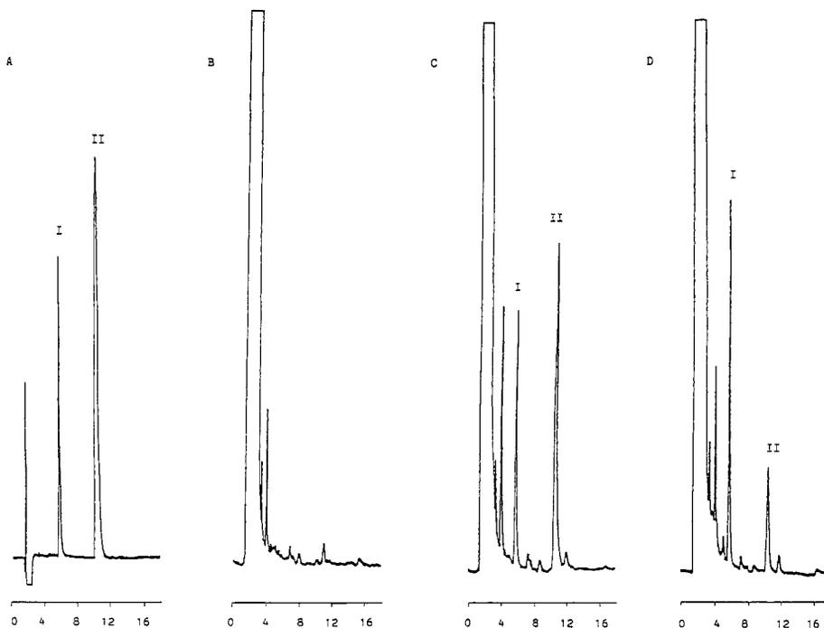
FIGURE 1. Typical chromatograms of the recovery of diclofenac (II) and naproxen (I) from aqueous standard diclofenac 1  $\mu\text{g/ml}$  naproxen 1  $\mu\text{g/ml}$  (A), plasma blank (B), plasma spiked with diclofenac 1  $\mu\text{g/ml}$  naproxen 1  $\mu\text{g/ml}$  (C) and plasma 80 minutes after an oral dose of 50 mg diclofenac (D).
