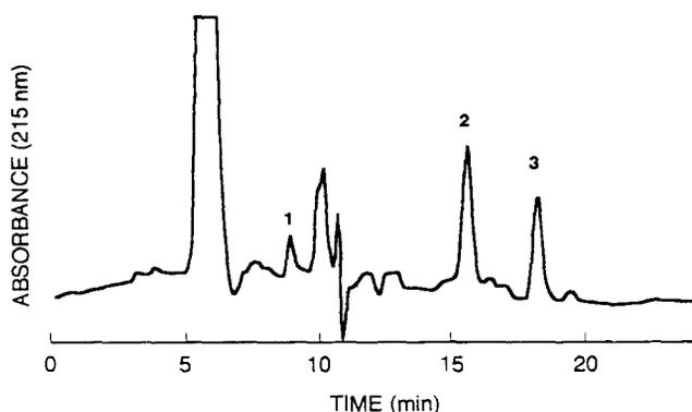
FIGURE 2. HPLC analysis of the crude extract of *L. lucidum* fruit. Mobile phase: methanol-water (9:1, v/v); flow-rate: 0.5 ml/min; detection 215 nm. Peak 1: unknown compound; peak 2: oleanolic acid; and peak 3: ursolic acid.
