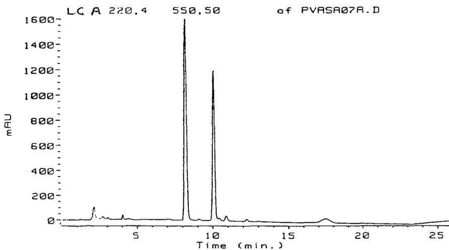
FIGURE 2: Analytical separation of *cis/trans* mixture (50  $\mu$ g)
