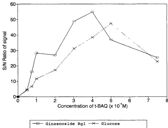
FIGURE 3. Effect of the concentration of t-BAQ on the peak response. conditions : 10W UV lamp with 45cm PTFE tubing; column : Lichrosorb  $\text{NH}_2$  column (250mm  $\times$  4mm i.d., 10 $\mu$ m); eluent : acetonitrile/water (80/20) with various concentration of t-BAQ; flow-rate : 1ml/min; reaction time : 4sec; detection : fluorescence (excitation : 400nm, emmission : 525nm).
