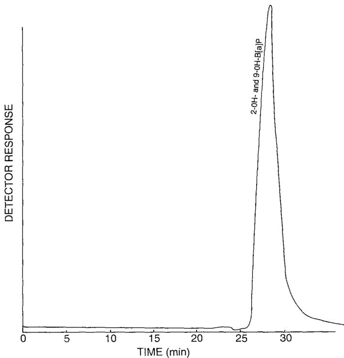
FIGURE 3. Chromatogram of 2-OH-B[a]P and 9-OH-B[a]P obtained with MeOH:H<sub>2</sub>O (80:20). The full names of the compounds are given in the footnote of Table 1.
