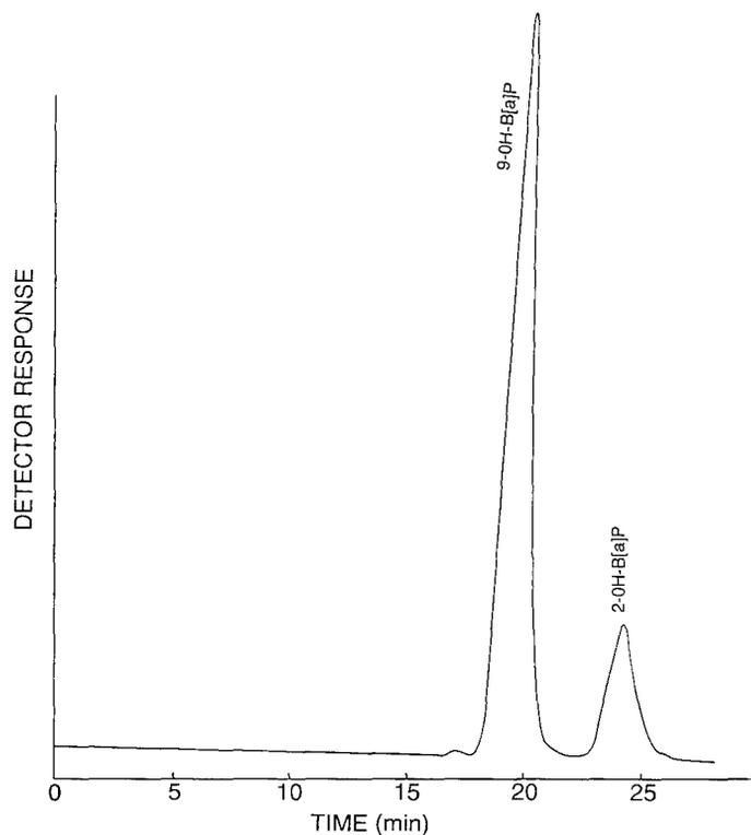
FIGURE 4. Chromatogram of 2-OH-B[a]P and 9-OH-B[a]P obtained in MeOH:H<sub>2</sub>O (80:20) with 1.7 mM  $\gamma$ -CD. The full names of the compounds are given in the footnote of Table 1.
