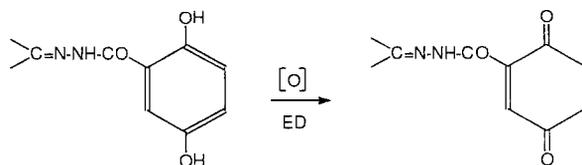
Scheme 2: General oxydative mechanism of electroactive Schiff bases **3 a-c** at porous graphite electrodes.
