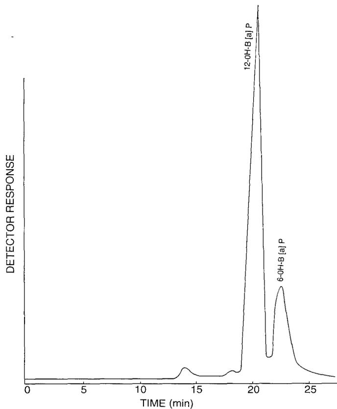
FIGURE 2. Chromatogram of 6-OH-B[a]P and 12-OH-B[a]P obtained in MeOH:H<sub>2</sub>O (75:25) with 3.5 mM  $\gamma$ -CD. The full names of the compounds are given in the footnote of Table 1. The smaller peaks in the chromatogram are due to impurities.
