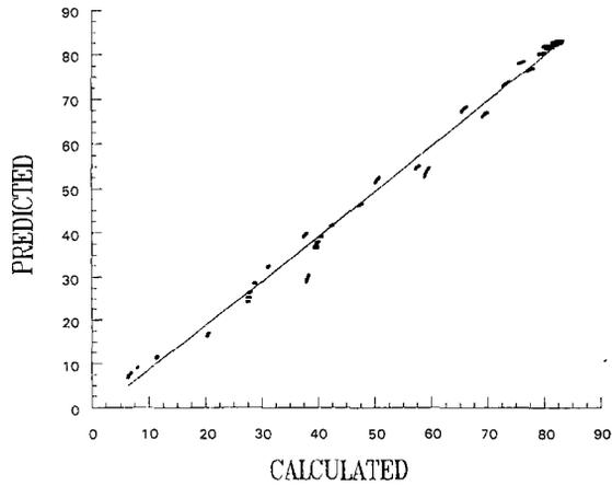
Figure 6. Plot of the neural network predicted and the actual calculated capacity factors when the network was trained with only 16 points and tested for 429 points ( $r=0.9969$ ).
