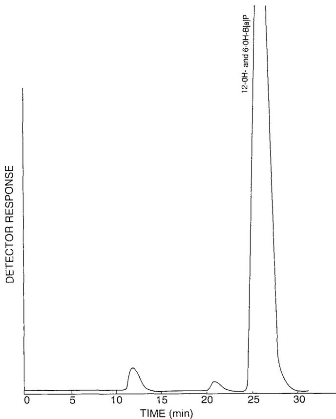
FIGURE 1. Chromatogram of 6-OH-B[a]P and 12-OH-B[a]P obtained with MeOH:H<sub>2</sub>O (75:25). The full names of the compounds are given in the footnote of Table 1. The smaller peaks in the chromatogram are due to impurities.
