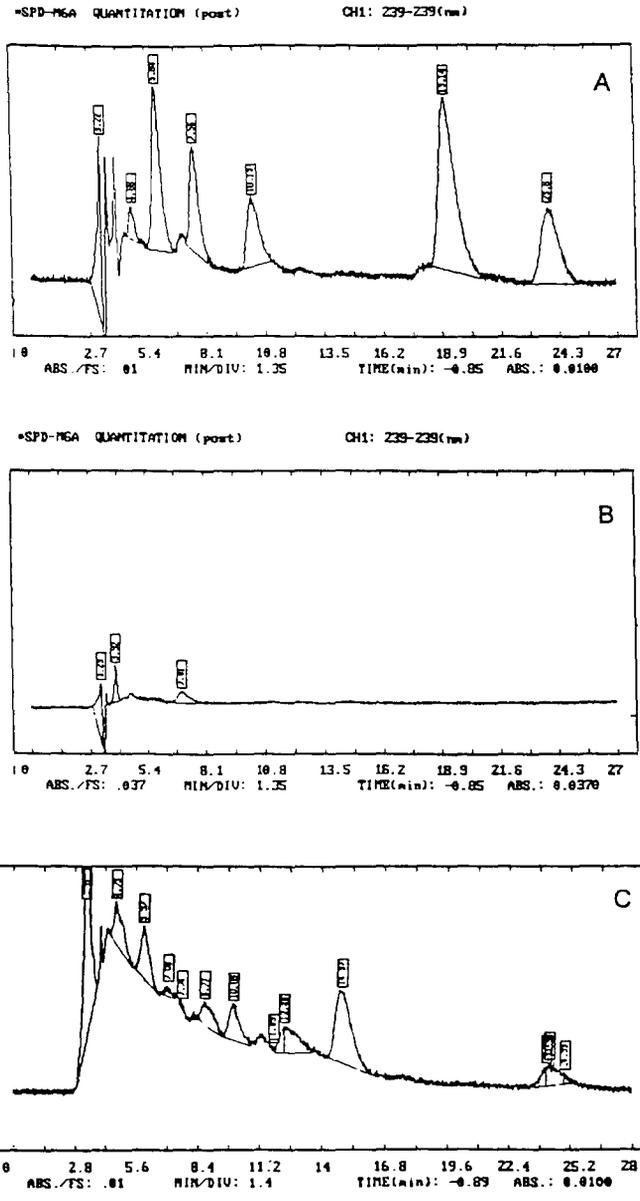
Fig. 3. A: Chromatographic analysis of urine spiked with morphine (5 ng/μl)=5.84 min, 6-MAM (5 ng/μl)=7.56 min, codeine (5 ng/μl)=10.19 min, papaverine (1 ng/μl)=19.14 min and the internal standard flufenamic acid (2.5 mg/ml)=25.8 min.
