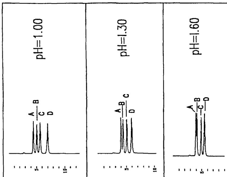
FIGURE 2. Effect of the pH of mobile phase on separation of A=(+)-acid; B=(-)-acid; C=(+)-ester; (D)=(-)-ester. The column temperature was 25°C and flow rate was 0.5 mL/min.
