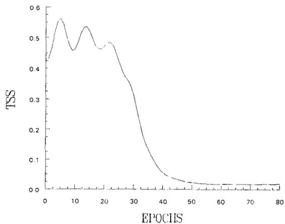
Figure 1b. Plot of the number of epochs and the corresponding tss when pH was the input and K was the target.
