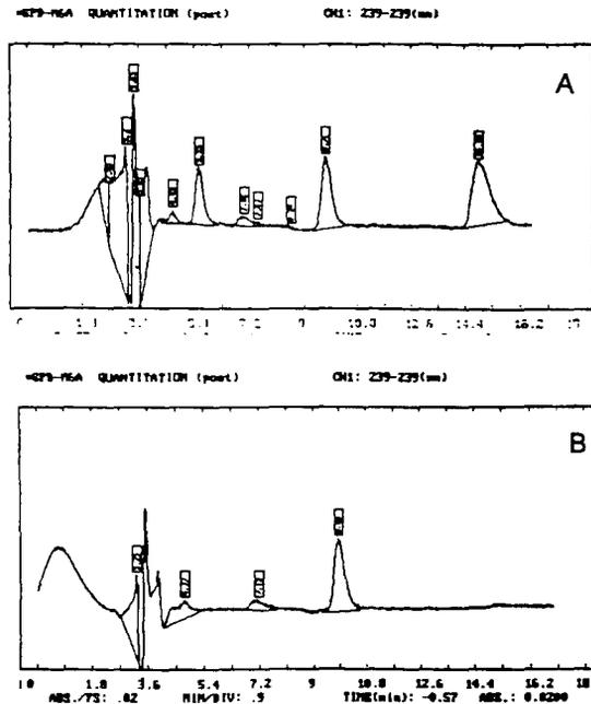
Fig. 2. (A) : Chromatographic analysis of plasma spiked with cocaine=14.55 min, benzoylecgonine=5.55 min and the internal standard naltrexone=9.72 min (at concentration 5 ng/μl for all the three compounds). (B) : Chromatographic analysis of blank plasma with the addition of the internal standard. Quantitation at 239 nm on both chromatograms.
