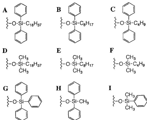
**FIGURE 1** Structures of the chemically bonded phases used in this study. (A)C18Diph, (B)C8Diph, (C)C4Diph, (D)C18, (E)C8, (F)C4, (G)Triph, (H)Diph and (I)Monoph.
