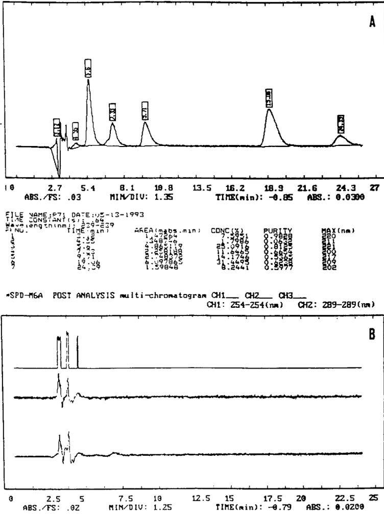
Fig. 1. A: Chromatographic analysis of plasma spiked with morphine (5 ng/ $\mu$ l)=5.6 min, 6-MAM (5 ng/ $\mu$ l)=7.33 min, codeine (5 ng/ $\mu$ l)=9.17 min, papaverine (1 ng/ $\mu$ l)=19.06 min and the internal standard flufenamic acid (2.5 ng/ $\mu$ l)=24.39 min. Quantitation at 239 nm. B: Chromatographic analysis of the same plasma sample prior to the addition of the alkaloids. Quantitation at 254 and 289 nm.
