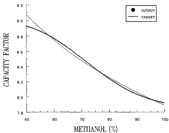
Figure 3. Plot of neural network trained output and calculated capacity factors reflecting the changes in methanol concentration in the mobile phase. ( $r=0.9935$ )
