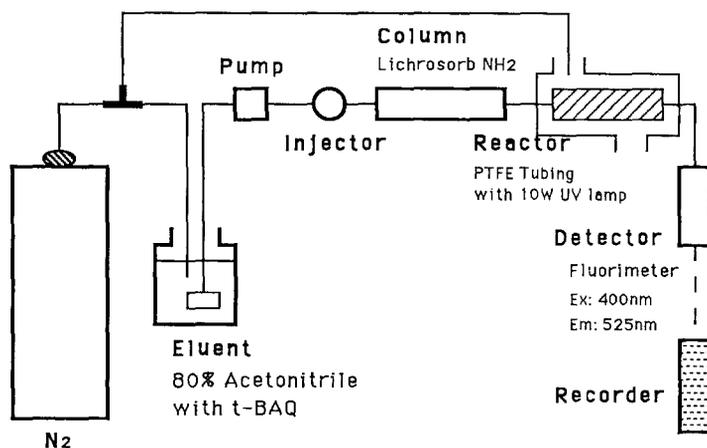
FIGURE 1. Scheme of photoreduction fluorescence detection system.
