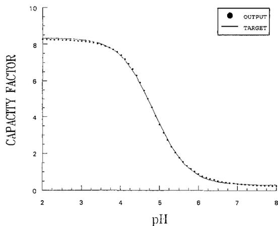
Figure 2. Plot of neural network trained output and calculated capacity factors reflecting the changes in pH of the mobile phase ( $r=0.9999$ ).
