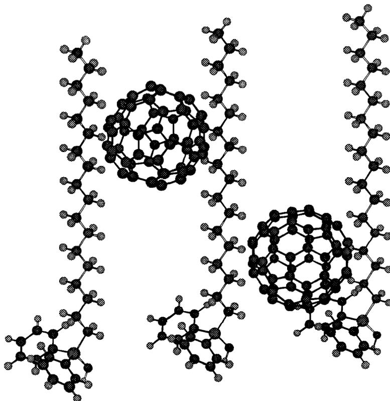
**FIGURE 4** Schematic diagram of the interaction between C<sub>60</sub> and the C<sub>18</sub>Diph bonded phase. The model was depicted by Chem3D Plus software (Cambridge Scientific Computing Inc., MA, USA). For convenience by the software, the bonded phase was drawn with hydroxyl group (-OH) as the residual functional substituent bonded to the silicon atom in the silanization reagent.
