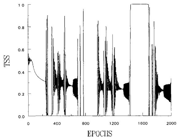
Figure 1a. Plot of the number of epochs and the corresponding tss when hydrogen ion concentration was the input and K was the output.
