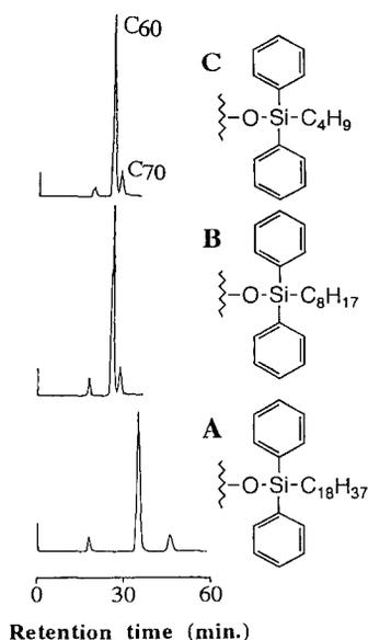
**FIGURE 2** Chromatograms for the separation of C60 and C70 with three alkyldiphenyl bonded phases. (A)C18Diph, (B)C8Diph and (C)C4Diph; mobile phase, n-hexane; column temperature, 30 °C.
