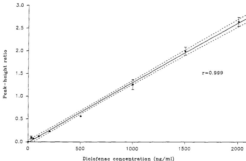
FIGURE 2. Calibration curve of diclofenac in human plasma.
