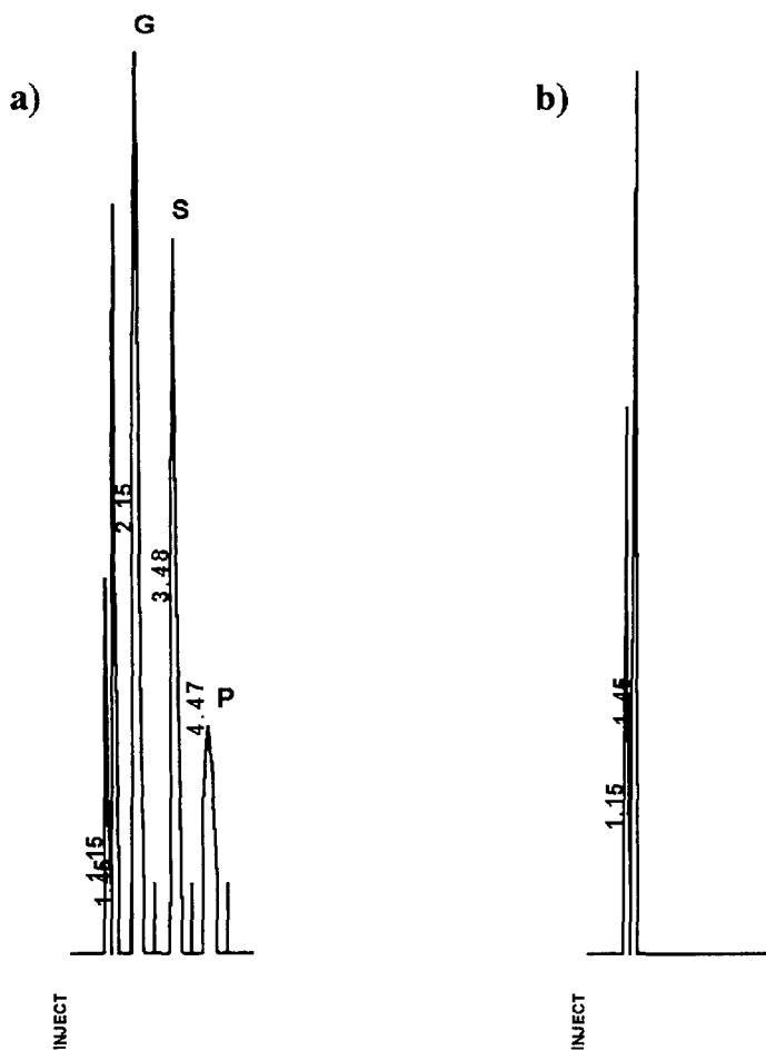
FIGURE 1. (a) Chromatogram of paracetamol (P) and its glucuronide (G) and sulphate (S) metabolites in urine. Concentrations P = 3.04 \mu\text{g mL}^{-1} ; S = 27.72 \mu\text{g mL}^{-1} ; G = 49.33 \mu\text{g mL}^{-1} . (b) Chromatogram of a processed urine blank.
