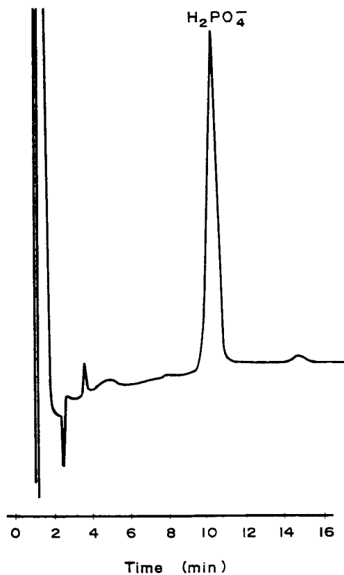
FIGURE 1: Chromatogram of a standard solution of dihydrogen phosphate (20 \mu\text{g}/\text{ml} ). Conditions: Water IC-Pak HR anion column with Sodium Borate/Gluconate pH = 8.5 eluent; conductivity detection; flow rate: 0.9 ml/min; injection volume: 100 \mu\text{l} .
