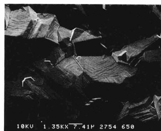
Fig. 4. SEM photograph of the surface of diamond film heat-treated at 650^\circ\text{C} for two hours.
