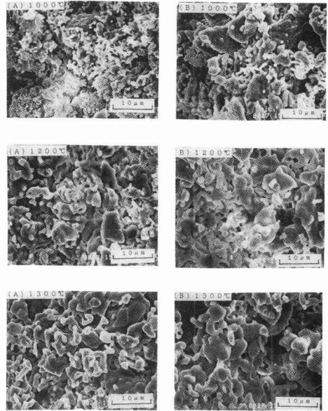
Fig. 6. SEM photograph of fracture surfaces of sintered sample (A) and (B) a various sintering temperatures.
