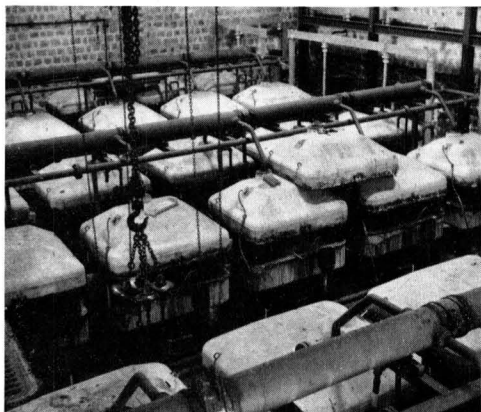
FIG. 1. Hooker "S" type caustic chlorine cells of The Mettur Chemical & Industrial Corporation Ltd., Mettur Dam, India.
