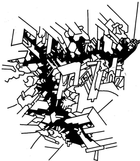
FIG. 7. Illustration of how regular mosaic crystal growth may occur in an alloy during freezing. Drawing represents primary lead dendritic branches enclosing pocket of near-eutectic composition into which extend numerous mosaic crystallites, lineages from the dendritic branches.
