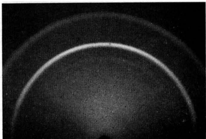
FIG. 2. X-ray diffraction photograph of nickel deposit formed in presence of 0.002 mole/l of ethylenediamine. No detectable preferred orientation.
