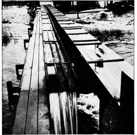
Running water troughs. For studying the action of sea water flowing at moderate velocities, specimens are immersed in the troughs, shown above. The total length of trough used for this purpose now amounts to about 600 feet.
