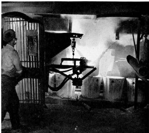
FIG. 4. Tapping an electric furnace at the Pacific Carbide and Alloys Company, Portland, Oregon.
