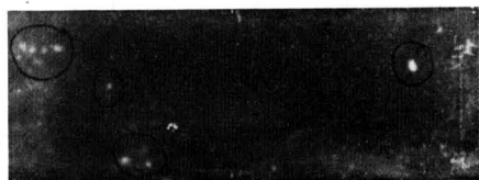
FIG. 1b. Radioautograph of steel coupon showing high concentration of radioactivity at circled spots. These spots are caused by adherent corrosion products. Exposure was to 3 \times 10^{-4}M chromate.
