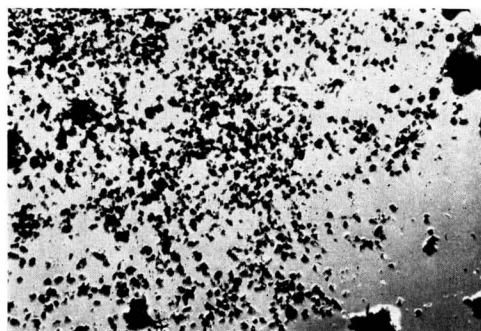
FIG. 10. Molybdenum powder from 100-gram batch produced at 600°C from bath B . 50X.
