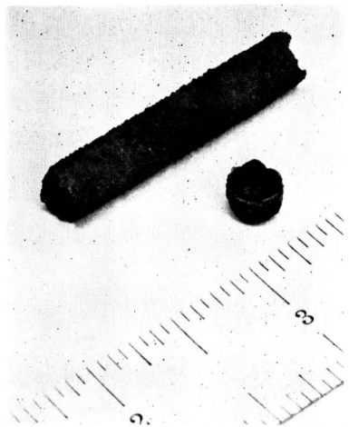
FIG. 9. Electroformed molybdenum tube and cup
