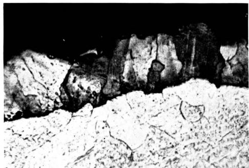
FIG. 4. Cross section of adherent molybdenum layer after removal of overlying powder—bath A. 500×
