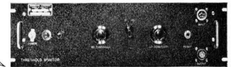
THRESHOLD MONITOR provides means for the control of voltage levels or rate of change.
