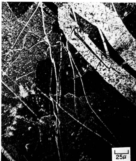
FIG. 3. Surface area from vertical wall of unequally cooled lead-antimony ingot containing 2% antimony. Original surface containing a few interdendritic and intergranular extrusions of antimony has been overrun by a molten stream of antimony-rich material originating at a mold face of lesser chill. Last formed film can be distinguished by its disregard for grain boundaries and other crystal structure. (Acetic acid-hydrogen peroxide etch.) 300X.
