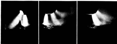
FIG. 2. Arc in a melting furnace. Three consecutive frames of a movie taken at a speed of 16 frames/sec.
