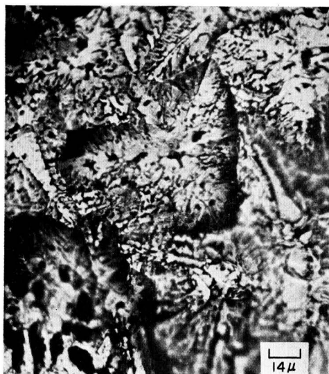
FIG. 2. Appearance at vertical surface of chill cast lead-antimony ingot after etch with acetic acid-hydrogen peroxide solution. Antimony (light areas) covers almost the entire surface and shows primary crystallization although representing only 5% of the total alloy. 500X.
