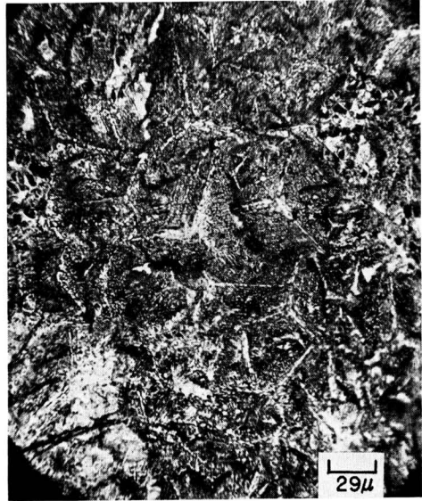
FIG. 9. A portion of the field of view to the left of the center of Fig. 4, considerably magnified. The tetrahedral shape of the individual crystals and the nature of the dendritic structure indicate oriented primary growth of antimony in the surface layer. 300X.
