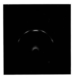
Fig. 27. X-ray photogram of rolled zirconium wire produced from electrolytic powder—MoK  $\alpha$  radiation.
