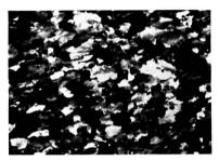
Fig. 24. Electrolytic zirconium metal, arc-melted and hot-rolled 80% from 0.375-0.07 in., at 700°C followed by 40% cold reduction from 0.070-0.030 in. Polarized light.
