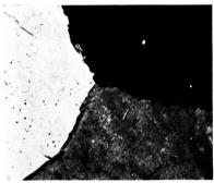
Fig. 31. Electrolytically produced zirconium metal, vacuum annealed 850°C for 5 hr, and furnace cooled. Hydride phase is still evident.  $150\times$
