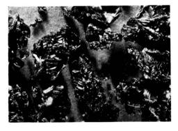
Fig. 8. As-recovered zirconium granules, water washed prior to compaction for arc melting. 15×
