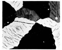
Fig. 28. Zirconium, vacuum annealed 2 hr at 800°C, furnace cooled, revealing hydride precipitation phase. Polarized light. 150×
