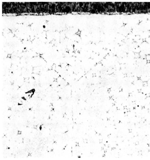
FIG. 1. Structure at surface of thorium reacted with nitrogen at 1370^\circ\text{C} . 250\times .
