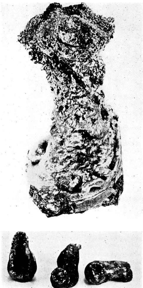
FIG. 3. Vermiculate \text{Be}_2\text{C} . Top—core of high-temperature heat; bottom—individual tubes showing hollowness.
