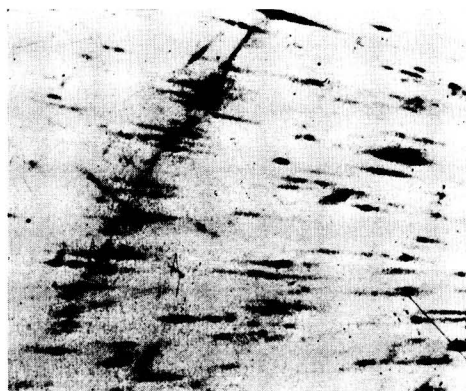
FIG. 1b. Enlargement of single-crystal spots from an arc pattern such as Fig. 1a.
